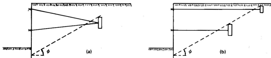
Fig. 35 – Typical anchorage for two tie rods
