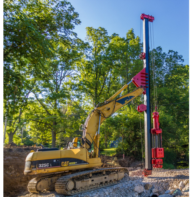
Figure 21. Excavator Mast Rig with Vulcan Impact Hammer (photo courtesy of Jonathan Tremmier, Vulcan Foundation Equipment)
