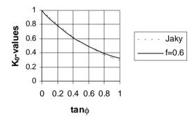
Figure 3. Earth pressure coefficient K<sub>0</sub>
