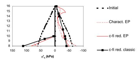
Figure 11. Earth pressures obtained by classic theory and FEM, Elasto-Plastic Model
