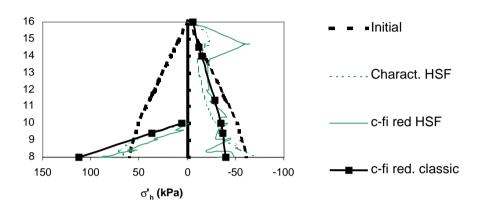
Figure 12. Earth pressures obtained by classic theory and FEM, Hardening Soil Model
