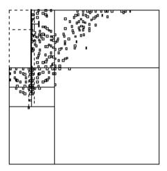
Figure 9. Pattern of plastified stress points at the end of c-fi reduction
