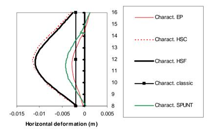
Figure 15. Horizontal displacements of the sheet pile wall, 6m excavation.
