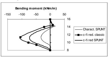
Figure 7. Bending moments obtained by SPUNT
