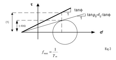
Figure 2. Shear mobilisation f ( $f=f_0$  at rest)
