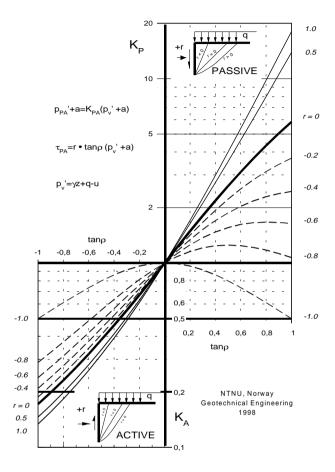
Figure 1. Earth pressure coefficients
