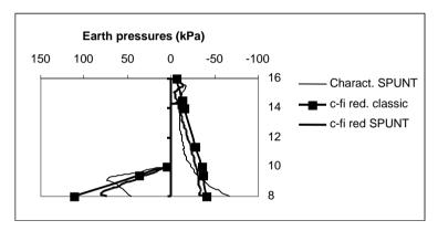
Figure 5. Earth pressures obtained by SPUNT
