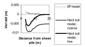
Figure 10. Ground deformations, fully excavated, no surface load
