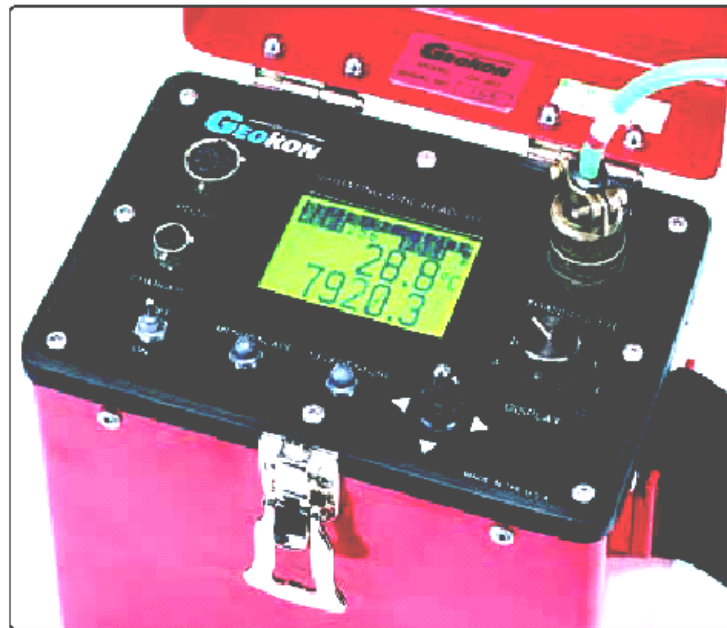
Figure 2.82 Model GK-603 vibrating wire readout box (website of Geokon, Inc.)
