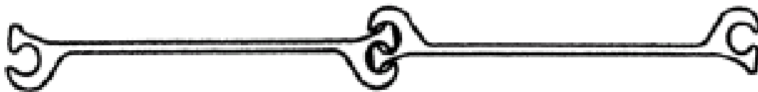
Figure 2.70 Typical configuration of straight or flat shaped steel sheet pile sections (website of Atlantic Sheet Pile, Inc.)
