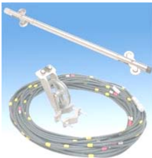
Figure 2.80 Inclinometer probe and cable (website of Geokon, Inc.)
