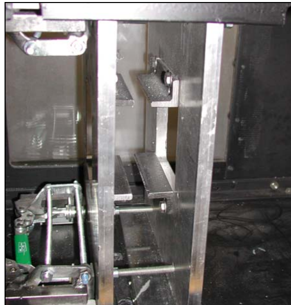
Figure 30. Specimen fixture for intermediate-velocity impact test.
