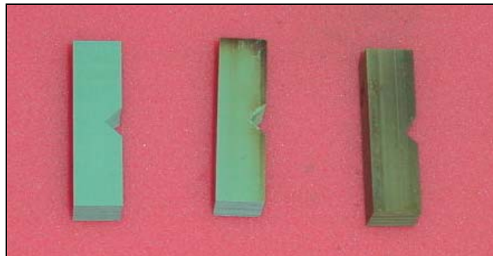
Figure 38. Izod test samples: unexposed (left), 20-hour exposure (center), 200-hour exposure (right).
