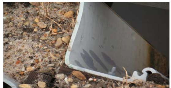
Figure 58. Examples of improper structural designing of PVC sheet pile showing buckling of the pile web, bending of the wall, and interlock failure.
