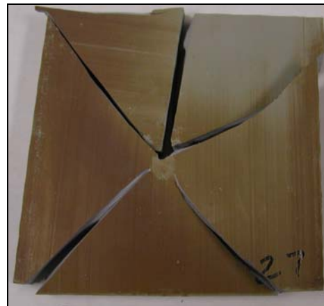
Figure 35. Intermediate-velocity impact damage in the PVC27 200-hour sample below the ballistic limit.
