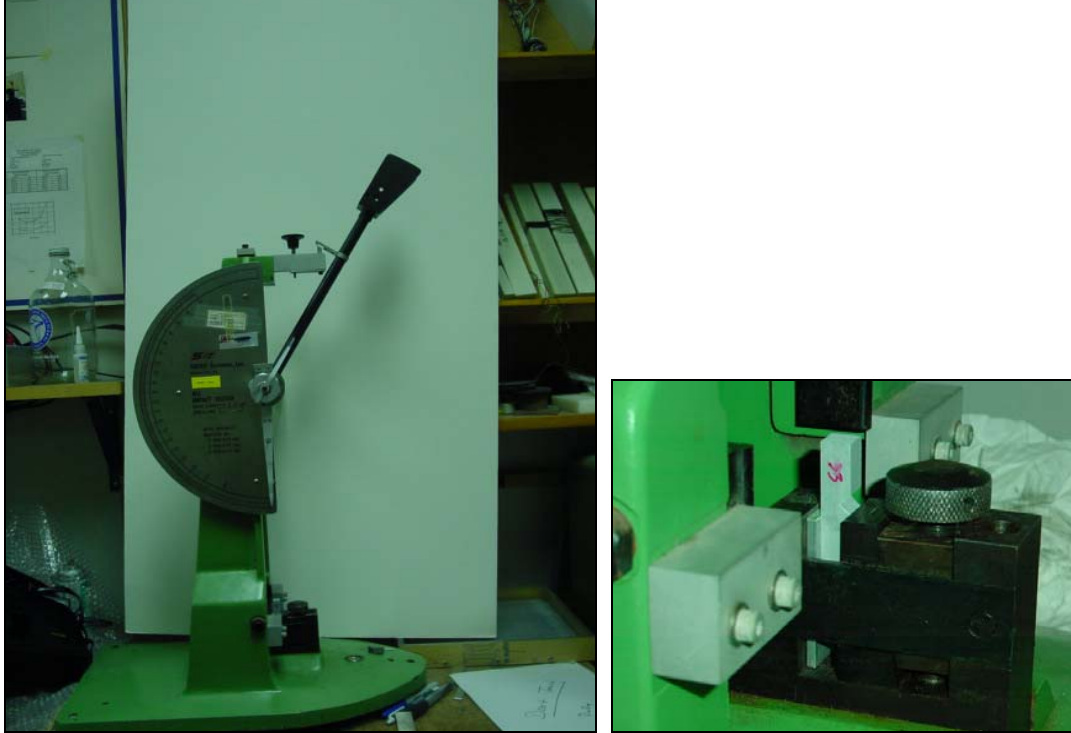
Figure 40. Izod testing machine with the samples shown in the anvil in the inset.
