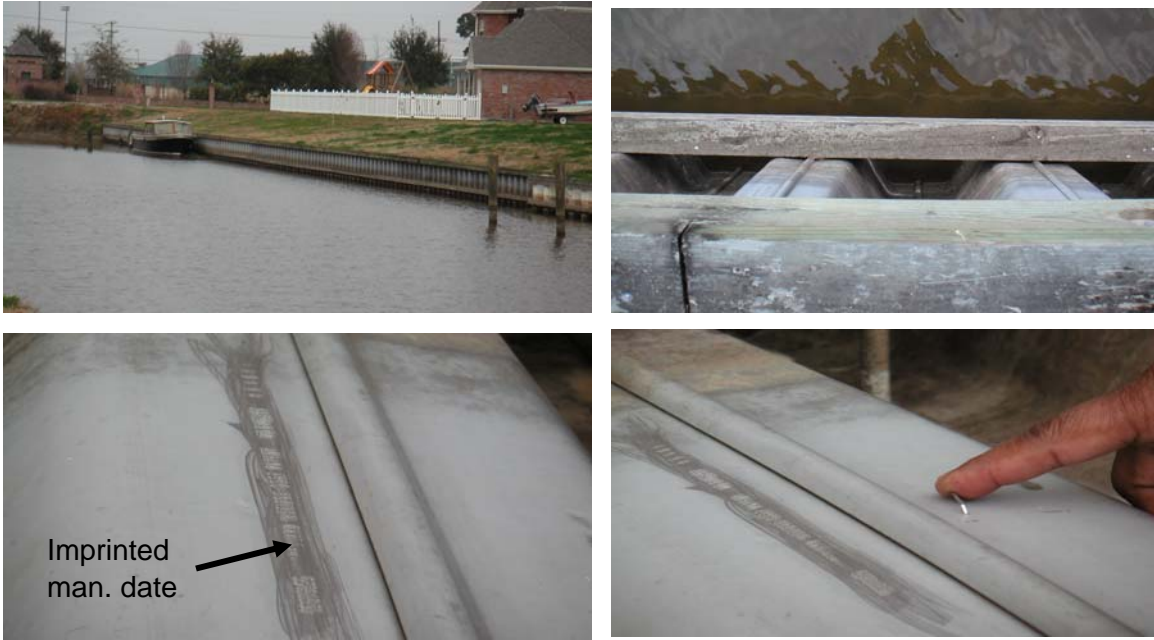
Figure 55. Ten-year-old sheet piling in Houma, Louisiana. Note the imprinted dates (left bottom) and staple gun impact test (right bottom) showing no cracks.
