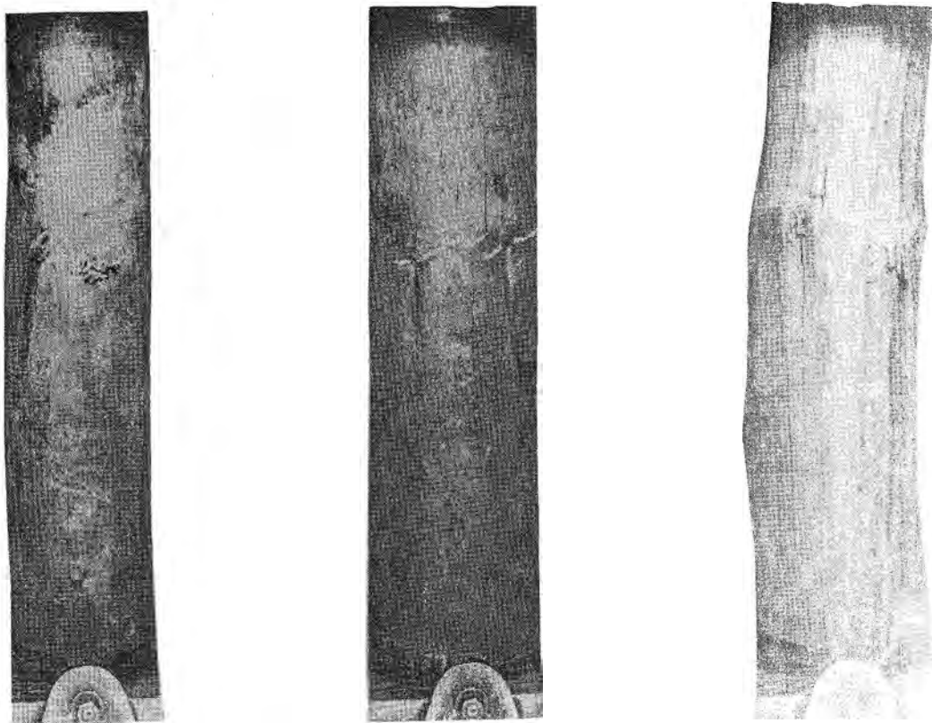
Figure 9.--Typical compression failures in tip sections of test piles: (left) southern pine, specimen P13; (center) Douglas-fir, specimen D10; and (right) red oak, specimen 02.
