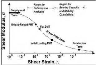
Figure 5. Typical Values of Shear Modulus Based on Field Tests (from Loehr, Lutenegger, Rosenblad, and Boeckmann (2016))
