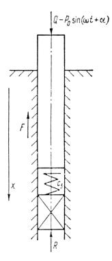
Figure 17. Vibratory model with toe elasticity (from Tseitlin et al. (1987))
