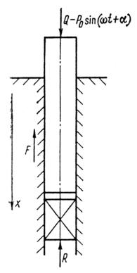
*Figure 3*. Computational diagram for vibrational driving using longitudinal vibrations (from Tseitlin et al. (1987))
