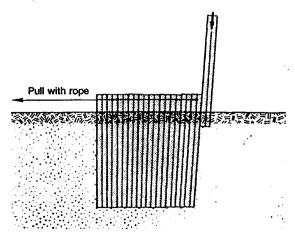
1.2.5. If the pile hammer is guided on a pile driving rig, fixed leader or swivel leader carefully press the leader against the sheet pile without exerting too much force.
