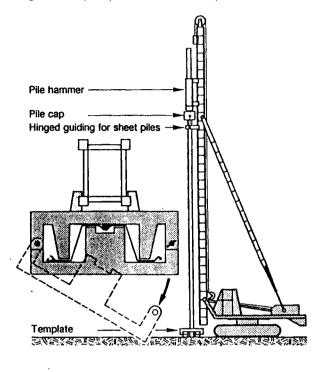
Driving very long sheet piles, it is recommended to use several pile guides. They prevent bending vibration, which leads to a considerable energy loss.
