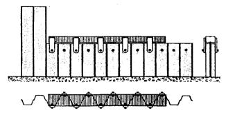
(This method is more complicated as the one described above, because the beam must be set ahead after each driven sheet pile). Weld interlocks together to prevent the moving of the adjoining sheet. If driving doubles weld the driven pair together at the toe.
