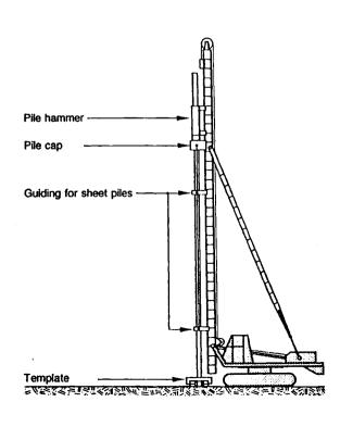
1.1.5. Driving sheet piles with swinging leaders, rope suspended leaders or free riding pile hammers, a frame type template should be used to guide the piles.
