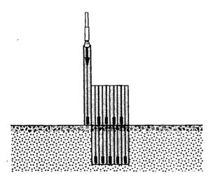
When driving sheet piles of uneven length weld stop blocks to the longer sheets.
