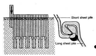
Sometimes it is sufficient to stop driving shortly above grade and drive the entire wall to grade later on.
