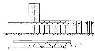
Install beam on top of the sheet wall and connect to the sheets via straps and bolts.
