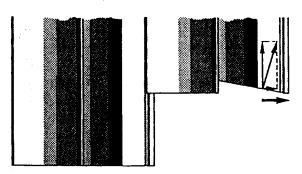
Note: Too much bevel can damage the pile.
