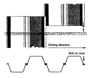
1.1.3. Make sure the pile hammer ist centered on the sheet pile, thus distributing the energy evenly to the pile.
