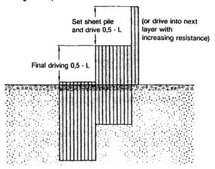
1.1.7. Driving cofferdams and cellular cofferdams, set and close the entire structure, then drive each 4th or 5th pile partially.
