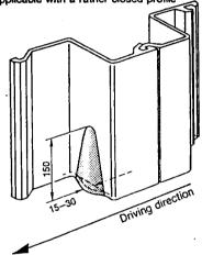
1.2.4. Take up all interlock play by pulling the last driven sheet against the direction of driving by means of one ore more "come-alongs".
