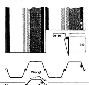
With Larssen sheet piles the leading interlock can be closed by a bolt or rivet of suitable size to enlarge the driving resistance at this point.
