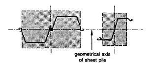
Driving a Larssen profile in single sheets and a \_\_\_\_\_\_ profile in doubles the pile cap does not cover the crossectional area evently.
