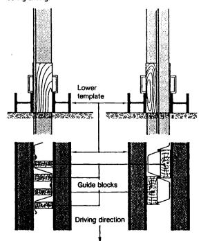
If for some reason it is not possible to use a guided pile cap, the sheets must be guided at the pile head by a pile guide to keep the pile centered under the pile hammer.
