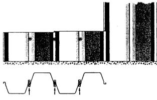
Install beams to each side of the sheet wall and fasten with holts
