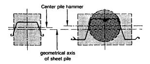
How much the pile hammer must be moved depends on the used profile and the friction in the interlocks.
