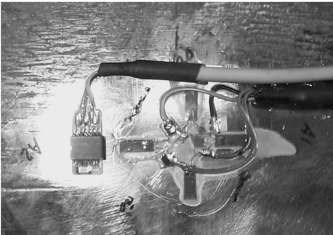
Figure 4-18 Accelerometer and strain-gauge circuit mounted on the inside of the web, near the sheet-pile head.
