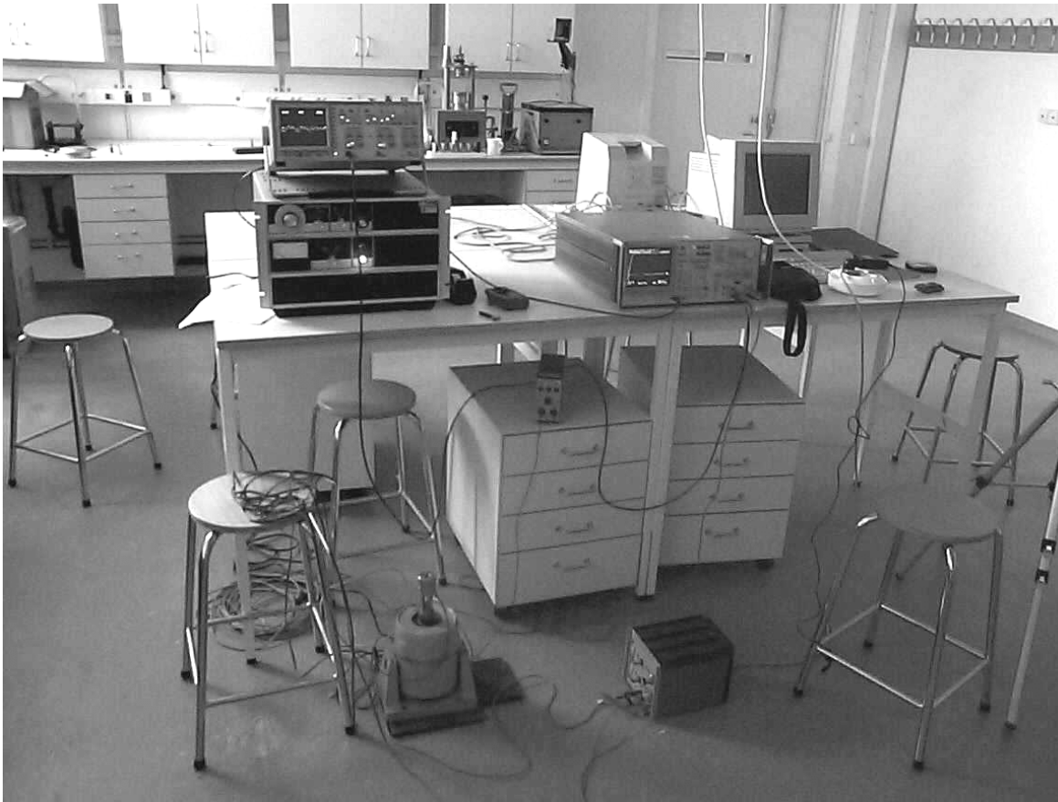
Figure 4-30 The calibration setup for the accelerometers. The power supply for the vibrator and the digital oscilloscope sitting above it can be seen on the left side of the workbench, and the HP frequency analyser can be seen to the right of these. The power supply for the accelerometer and the vibrator can be seen on the floor, and the amplifier for the reference accelerometer can be seen sitting on top of the chest of drawers under the bench.
