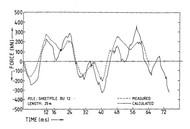
Fig. 13: Comparison Measured and Calculated Force-time diagrammes
