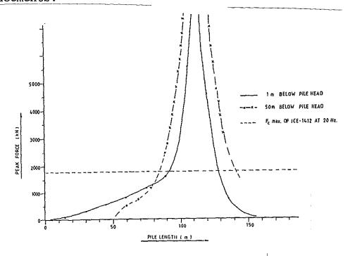
Fig. 11: Max. Peakforce vs Pile length
