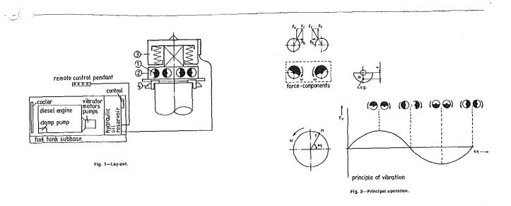
The pairs (one or more) of counter-rotating eccentric masses rotate usually at frequencies (f) between  $20-30~{\rm Hz}$  ( $1200-1800~{\rm cpm}$ ).
