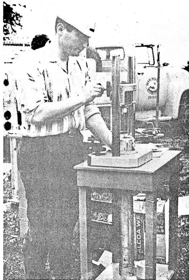
Figure 6.3. Performing vane shear test at field site.
