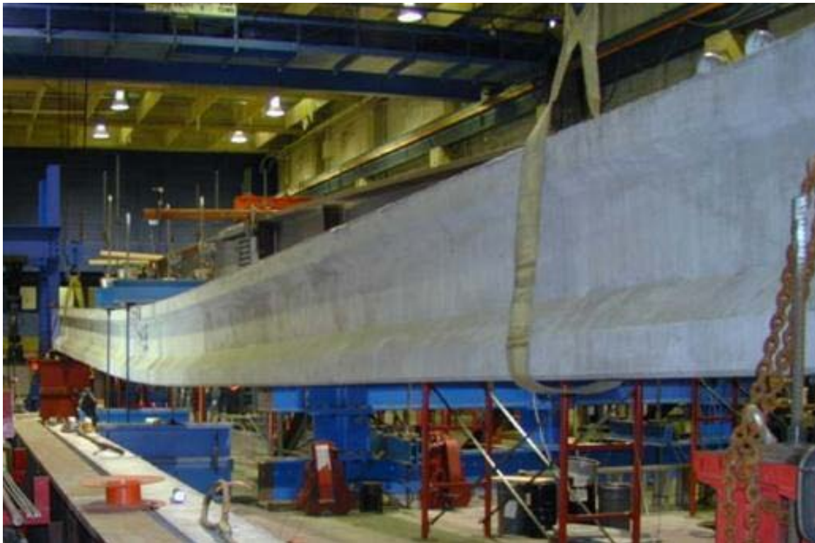
Figure 2.28. An 80-ft (24-m) girder with 17 in. (430 mm) of deflection (Graybeal 2005)
