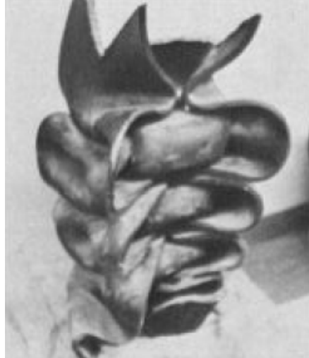
Figure 1.6. Lower portion of steel H-pile driven into Alaskan permafrost with an impact hammer (Huck and Hull 1971)
