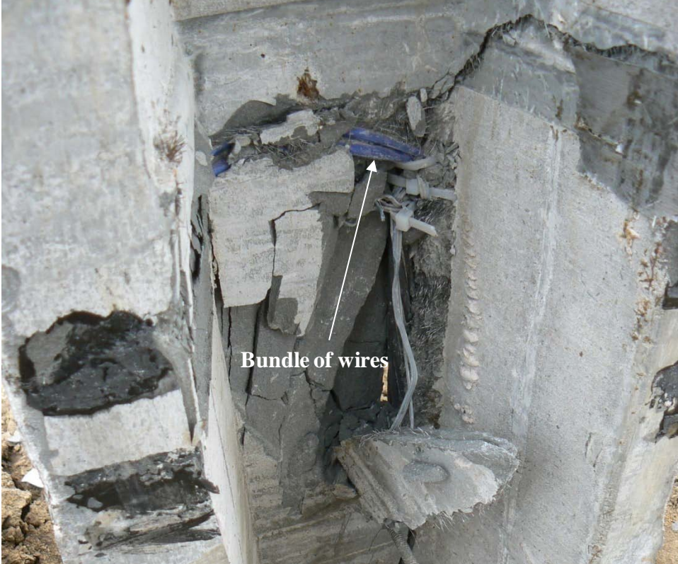
Figure 5.49. Shear failure region of UHPC pile P1 after the lateral load test with some cracked UHPC pieces removed
