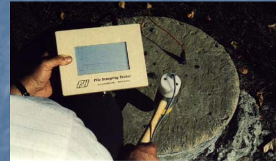
PIT (Pile Integrity Test)
