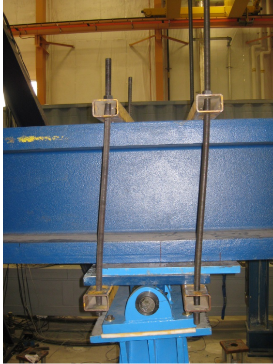
Figure 51: Movement of Saddle at Loading Point After Failure
