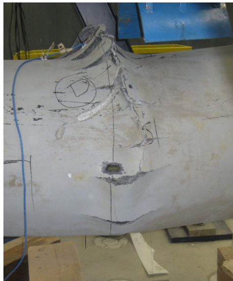
Figure 40: Compression Failure of Pile C-8HFB
