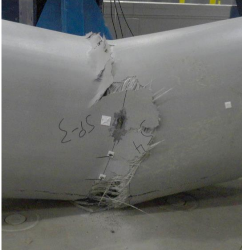
Figure 31: Tension Failure of Pile E-4FB
