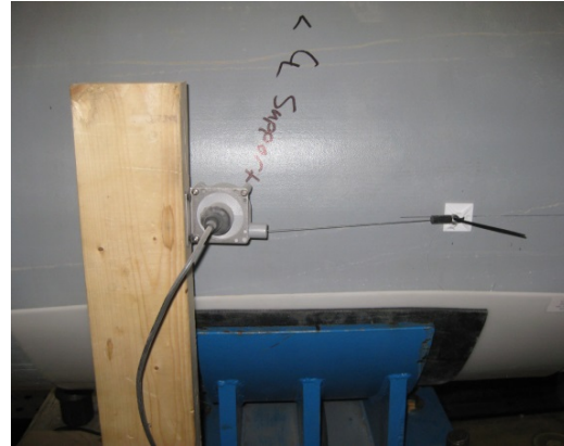
Figure 8: Lateral Translation Measurement
