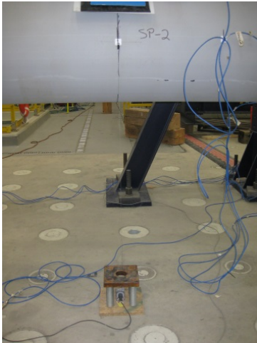
Figure 7: Vertical Deflection Measurement
