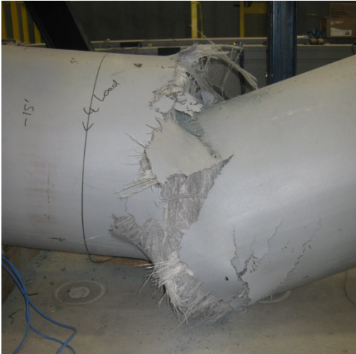
Figure 21: Tension Failure of Pile G-4FB
