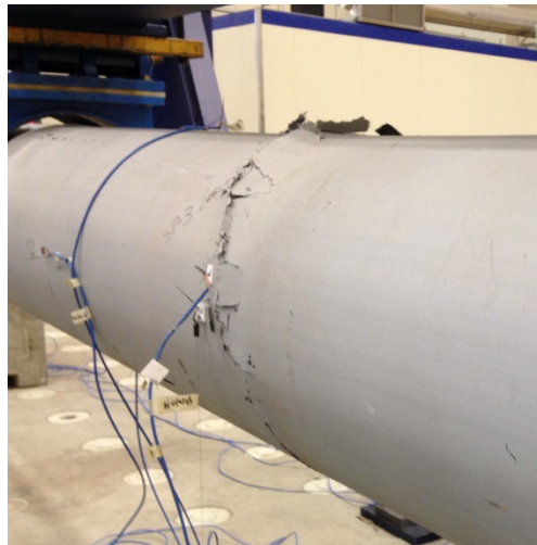
Figure 13: Compression Failure of Pile J-8HB
