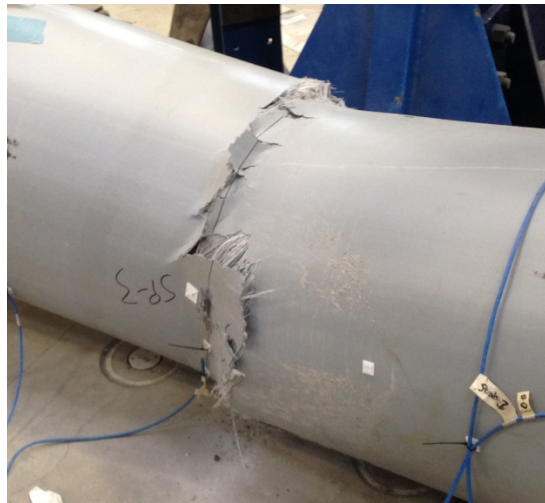
Figure 33: Tension Failure of Pile F-4FB
