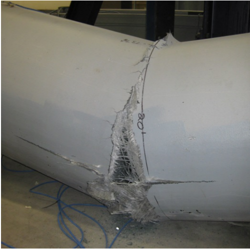
Figure 23: Tension Failure of Pile H-4FB
