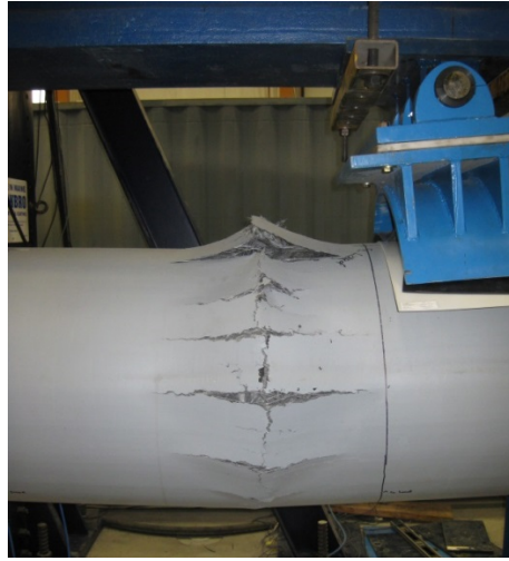
Figure 12: Compression Failure of Pile I-8HB
