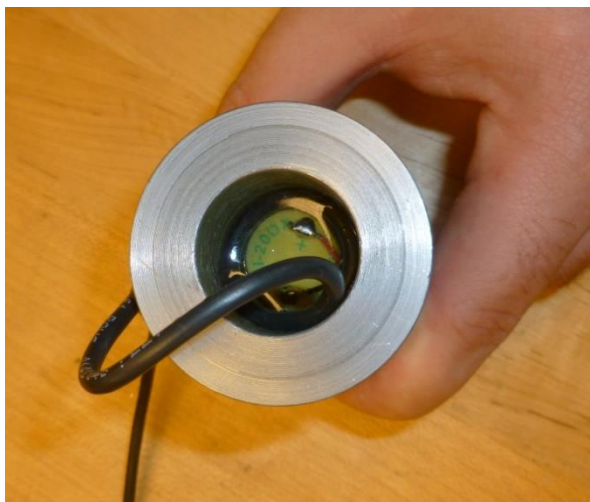
Figure 2-6 Geophone potted in push cone
