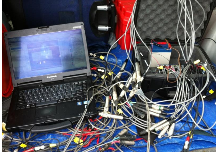
Figure 2-8 Data acquisition system and laptop
