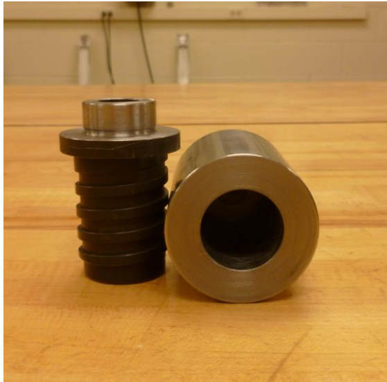
Figure 2-4 Cone and push adaptor
