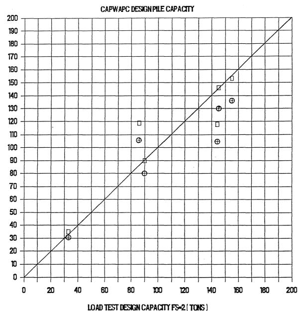
CALCULATED DESIGN CAPACITY (TONS)
