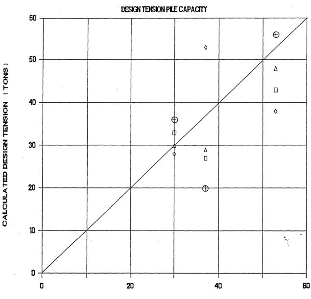
LOAD TEST DESIGN CAPACITY FS-2 (TONS)
