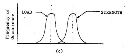
Load and Strength Distributions with Frequency of Failure
