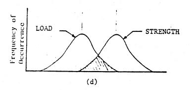
Effect of Variability on Frequency of Failure
