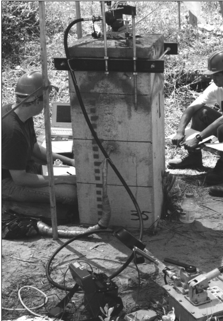
Figure 19.4 Osterberg Test in Progress on a 457 mm Concrete Pile (courtesy of Loadtest, Inc.)
