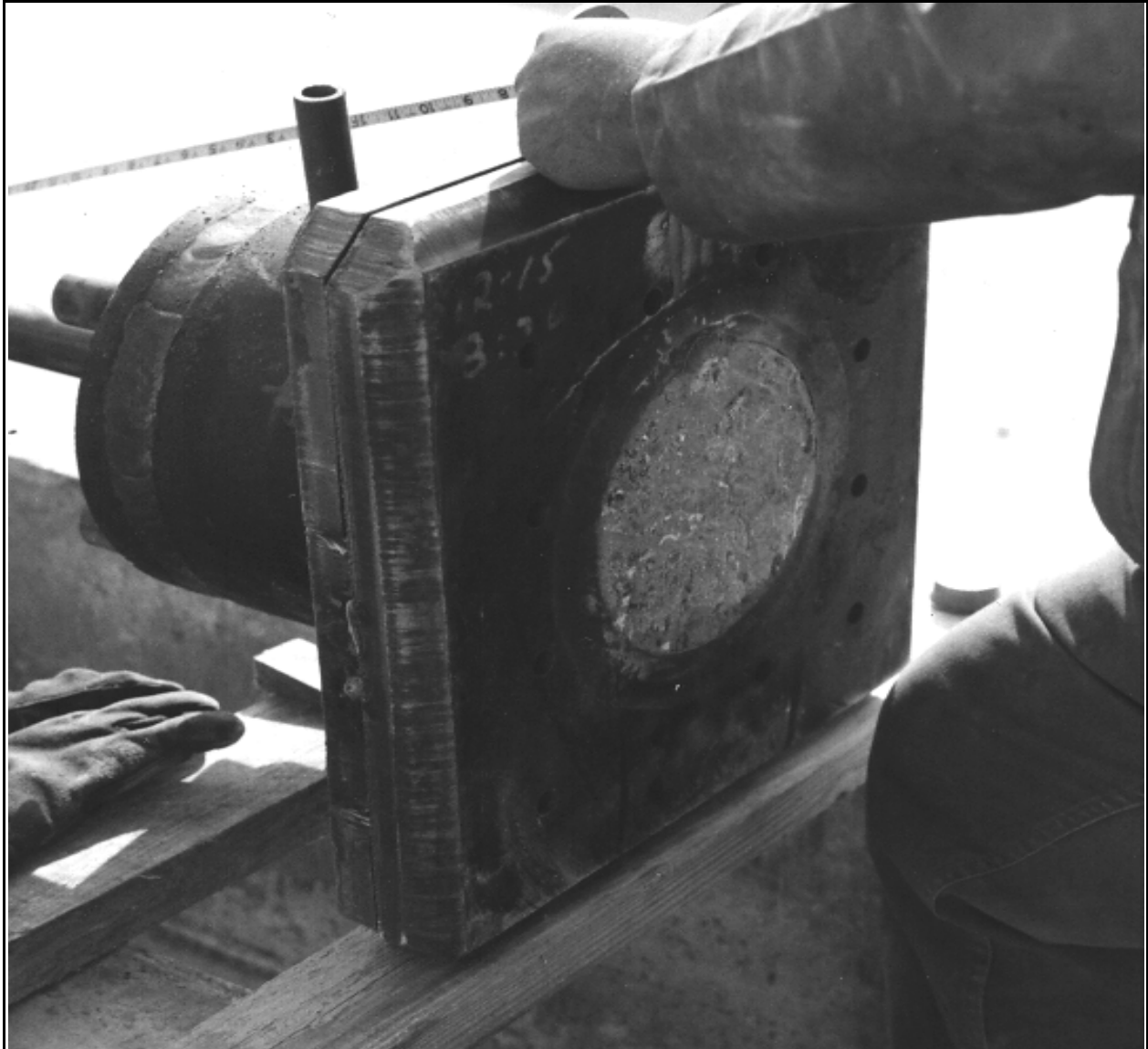
Figure 19.3 Osterberg Cell Ready for Placement in Concrete Pile Form (courtesy of Loadtest, Inc.)
