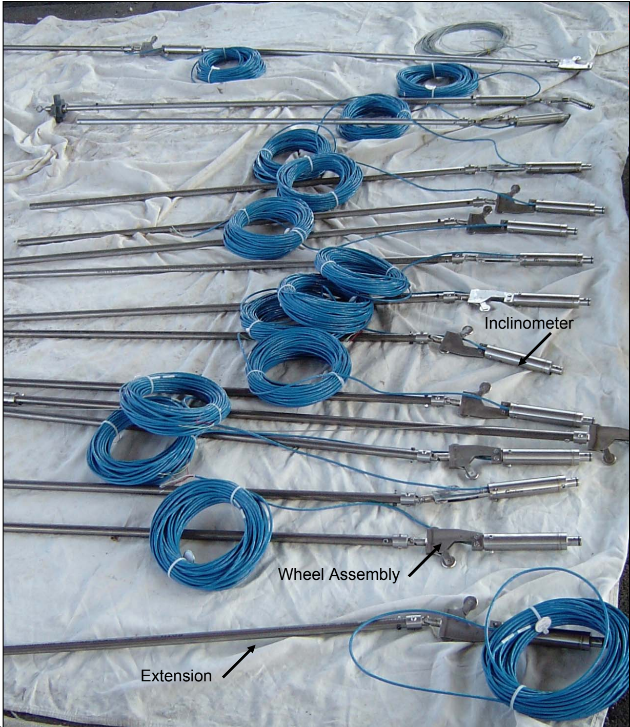
Figure 18.16 Multiple Incliner String Components for Lateral Load Test
