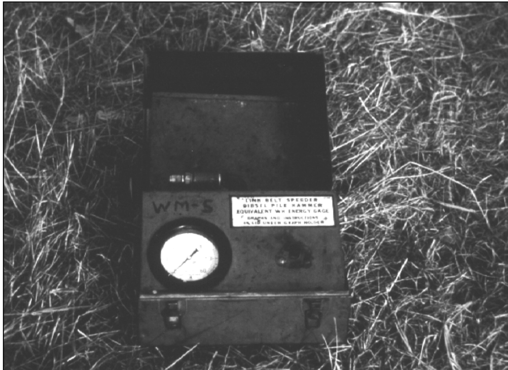
Figure 23.12 Typical External Bounce Chamber Pressure Gauge
