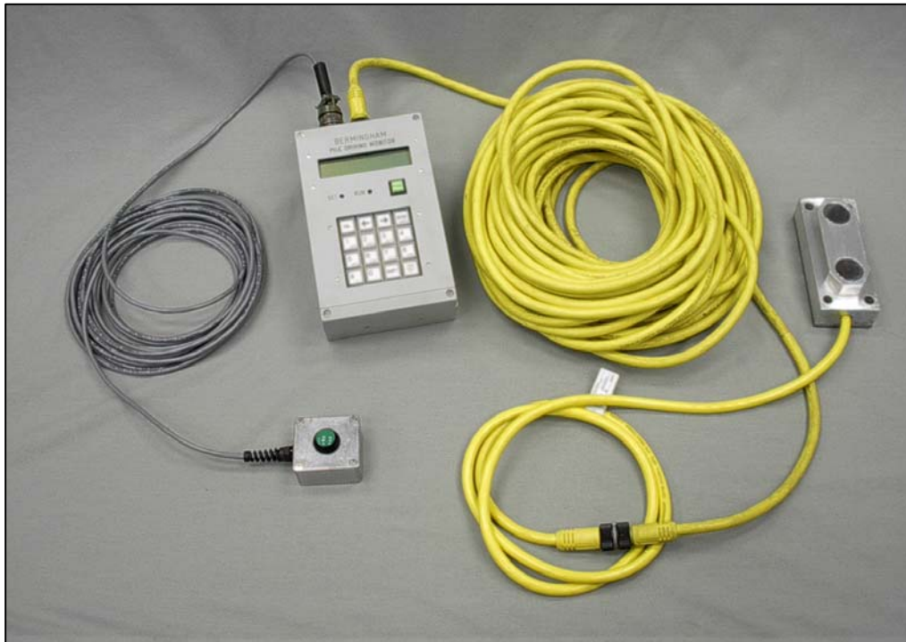
Figure 21.29 Proximity Switches, Readout Device, and Driving Log Trigger Switch for Berminghammer Diesel Hammer
