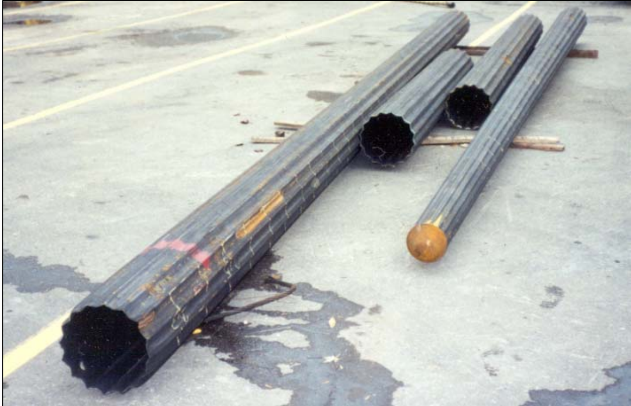
Figure 8.12 Tapered Monotube Section With Add-on Sections
