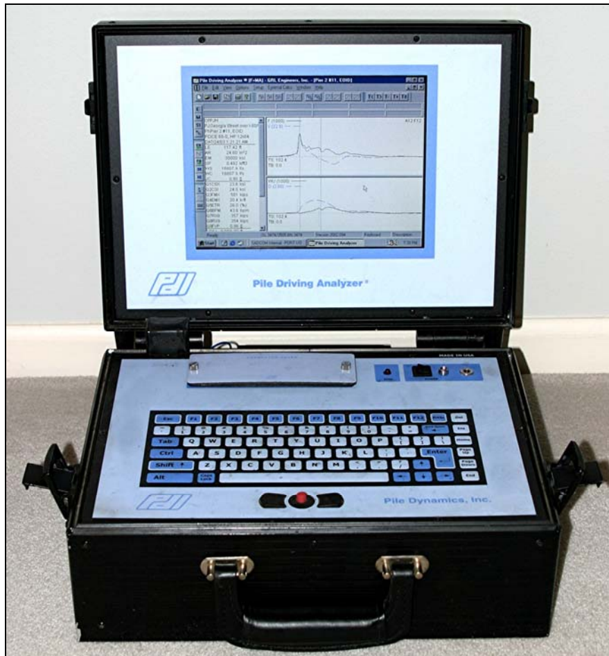
Figure 17.4 Pile Driving Analyzer – Model PAK (courtesy of Pile Dynamics, Inc.)
