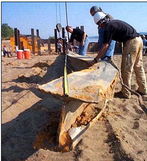
Figure 17.26 Photographs of Extracted Damaged Pile From Figure 17.25
