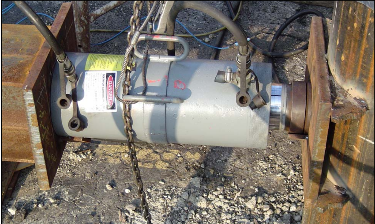
Figure 18.14 Jack for Lateral Load Test (courtesy WKG2)
