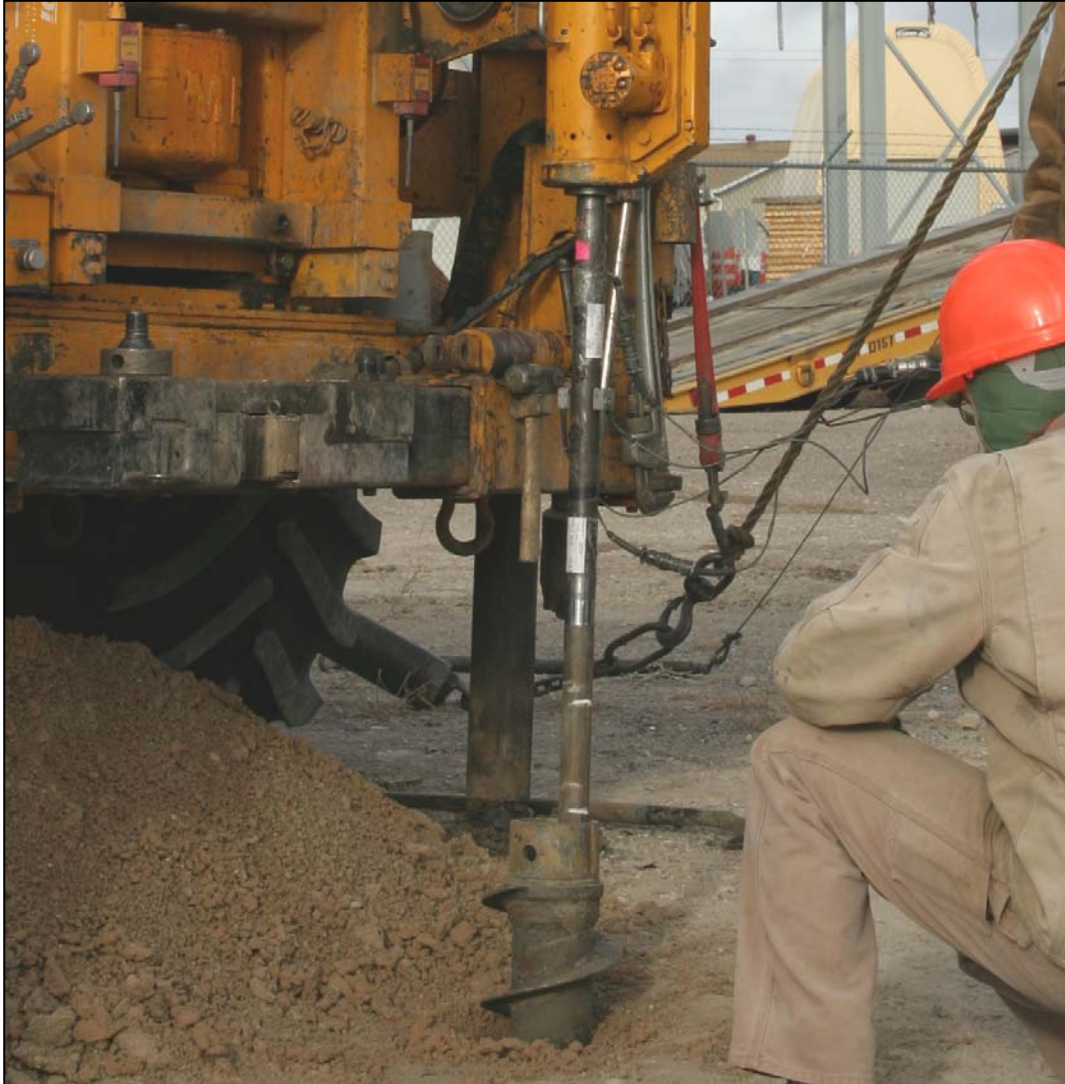
Figure 4.4 Energy Measurements on Automatic SPT Hammer
