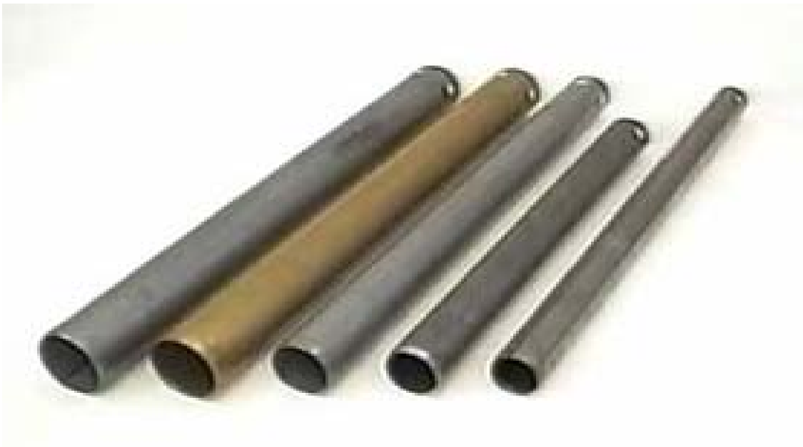
Figure 4.7b Various Diameter Shelby Tubes from Mayne, et. al., (2002)
