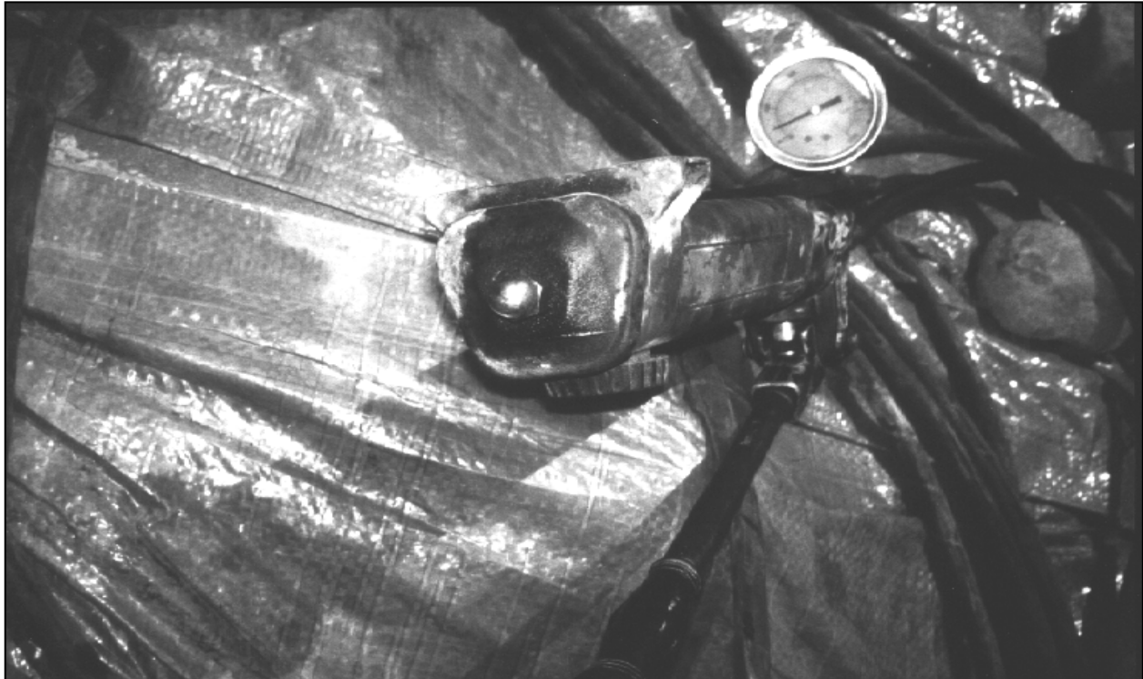
Figure 23.10 Adjustable Pressure Pump for Fuel Setting on ICE Hammer
