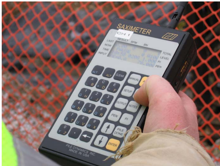
Figure 21.31 E-Saximeter Wireless Kinetic Energy Readout Device
