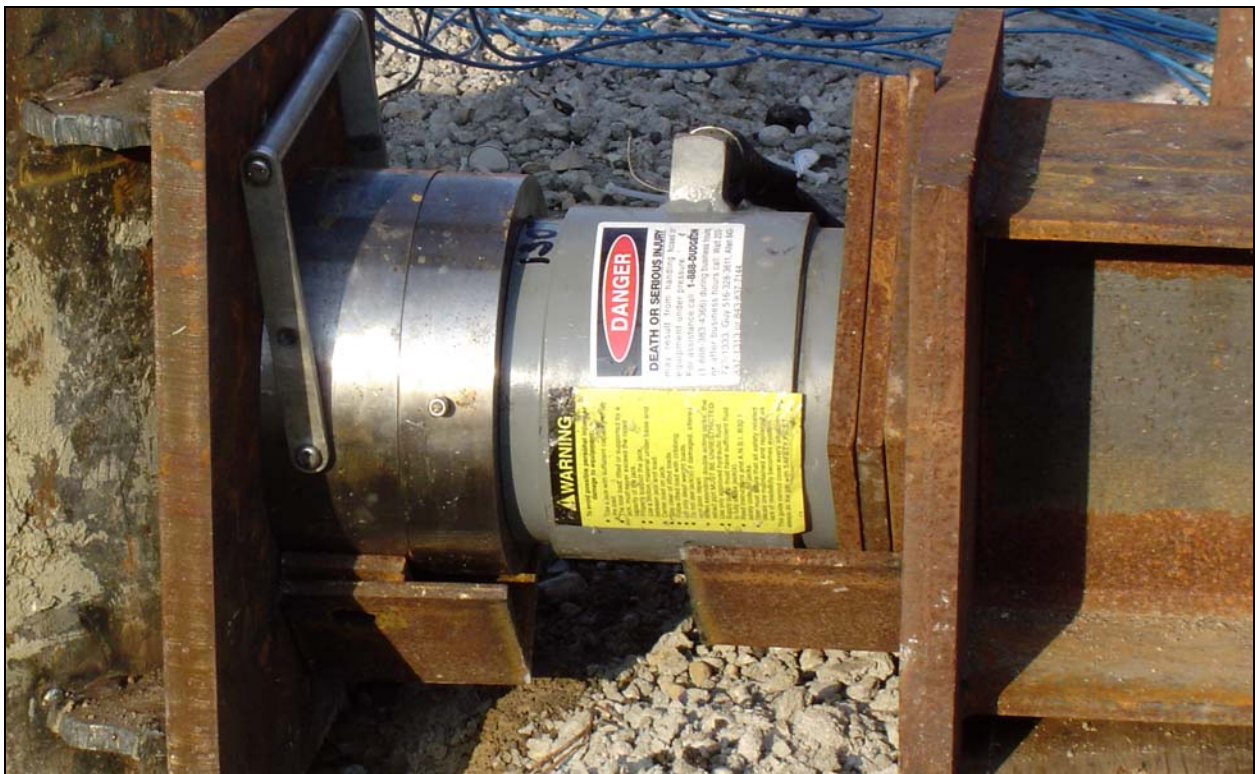
Figure 18.15 Spherical Bearing Plate and Load Cell for Lateral Load Test
