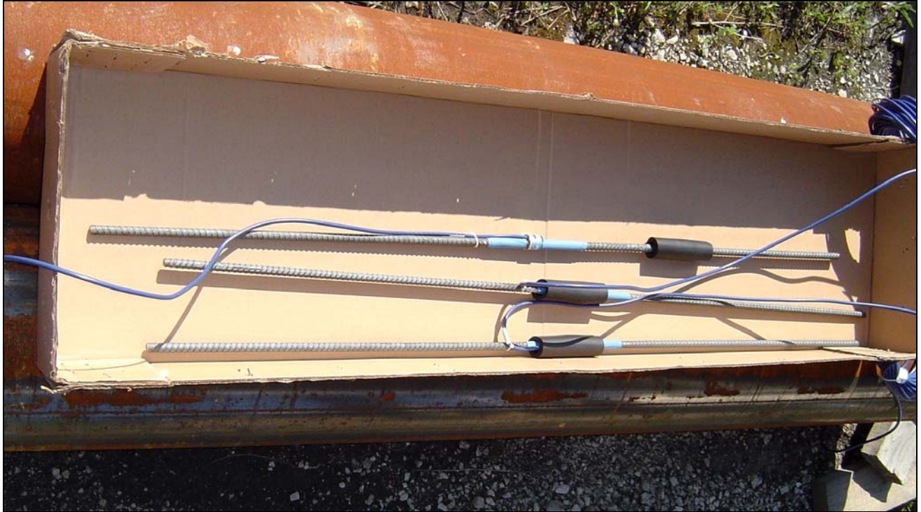
Figure 18.9 Sister Bar Vibrating Wire Gages for Concrete Embedment
