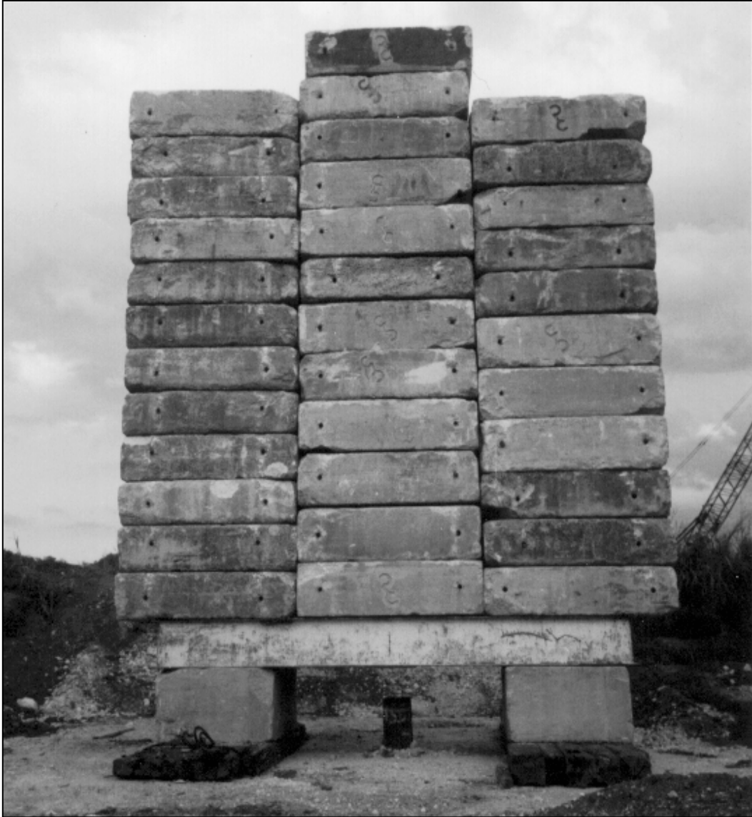
Figure 18.6 Typical Compression Load Test Arrangement using a Weighted Platform
