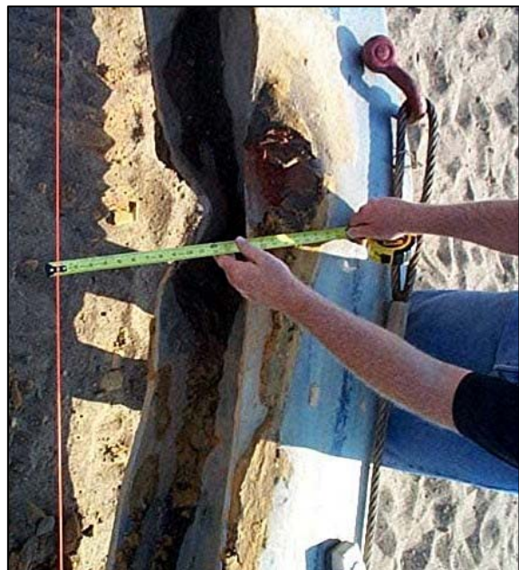
Figure 17.26 Photographs of Extracted Damaged Pile From Figure 17.25
