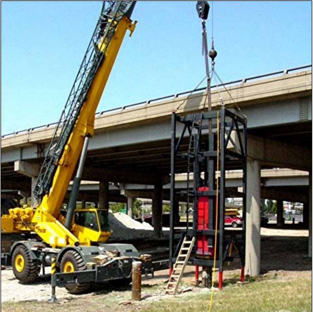
Figure 17.20 APPLE Drop Weight System (courtesy GRL Engineers, Inc.)
