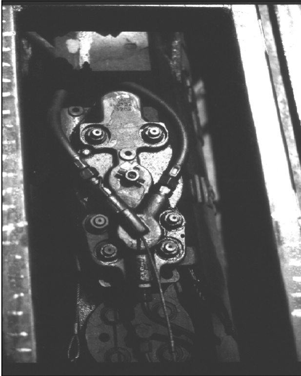
Figure 23.8 Fixed Four Step Fuel Pump on Delmag Hammer
