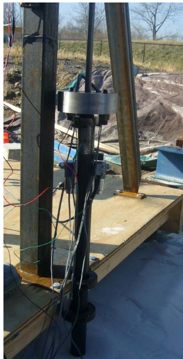
Figure A.10 Close-up on drop hammer and model pile top
