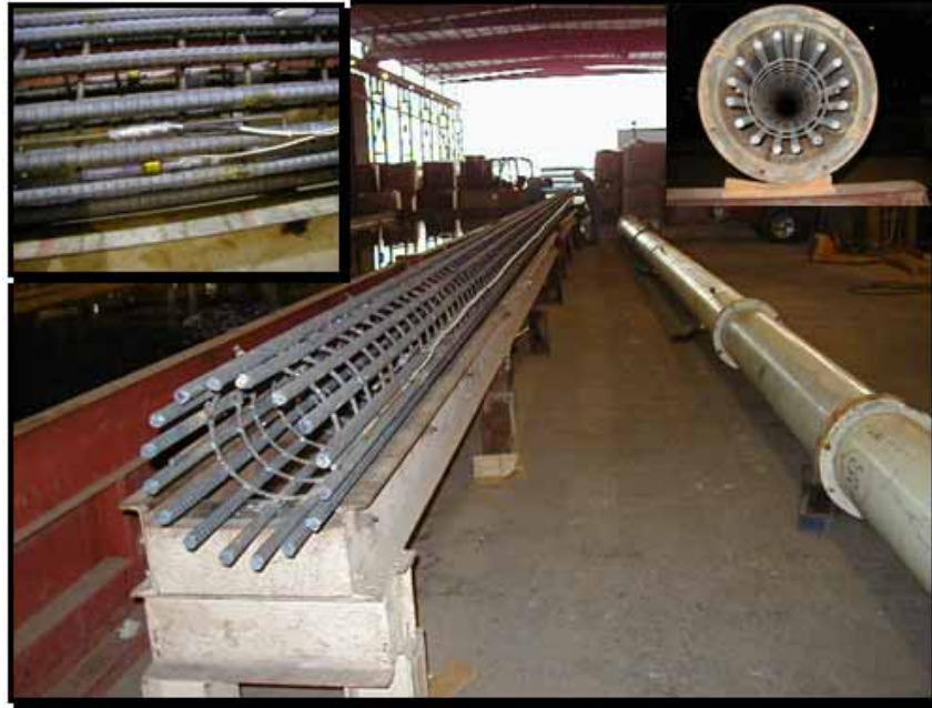
Figure 44. Photo. Vibrating and foil strain gauges attached to steel cage in PPI pile.
