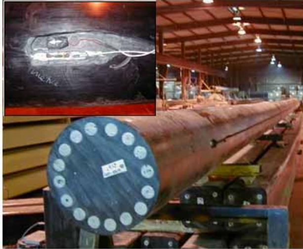
Figure 45. Photo. Vibrating and foil strain gauges attached to SEAPILE composite marine pile.
