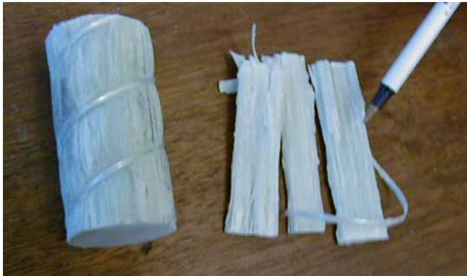
Figure 11. Photo. Fiberglass bar before axial compression test and disintegrated fiberglass parts.
