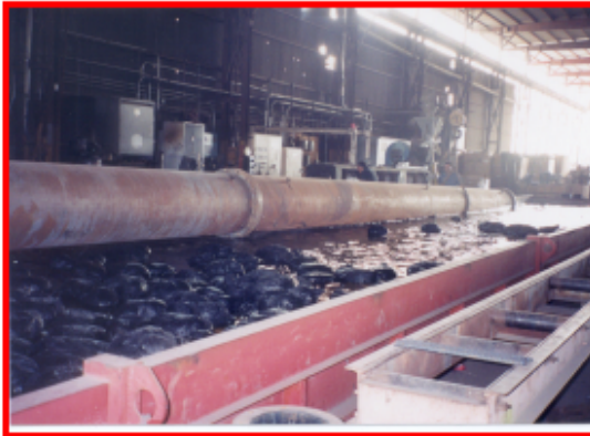
c) Mold submerged in cooling tank
