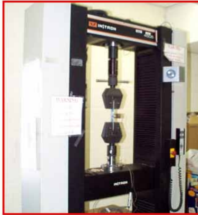
Figure 40. Photo. Typical tension test setup.
