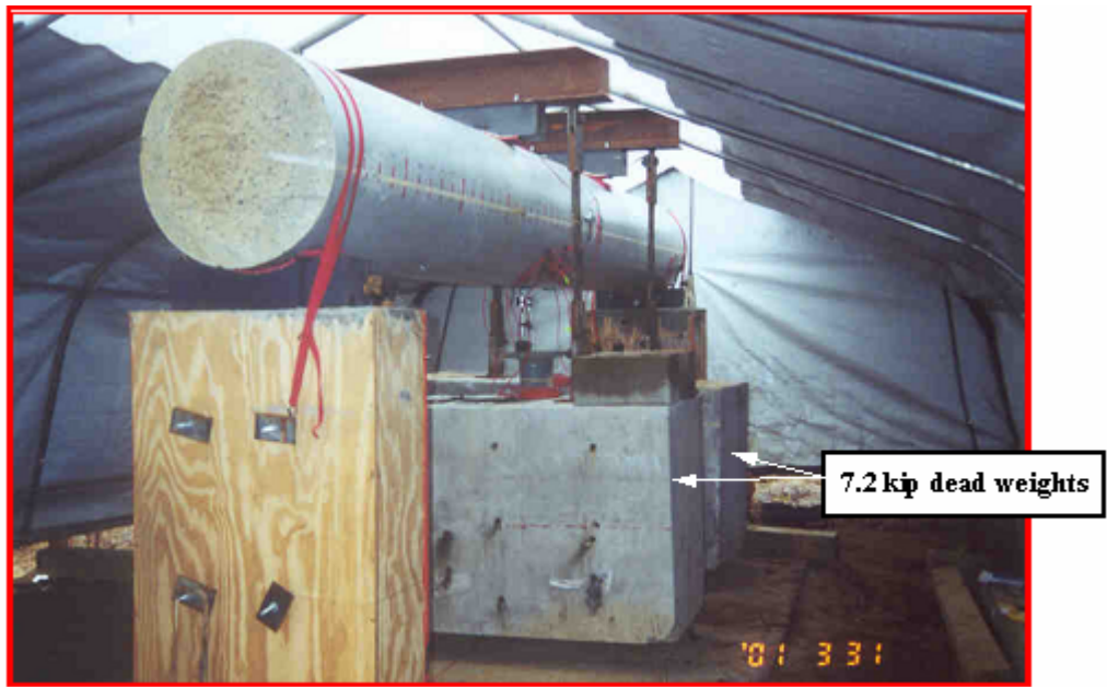
Figure 239. Photo. Creep bending test setup.
