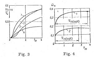
Fig. 3. Effect of packing length on rebound velocity of the ram for values of  $A_{mk}$  equal to 1)  $A_{13} = 6$ ,  $A_{23} = 0.06$ ; 2)  $A_{13} = 6$ ,  $A_{23} = 0.14$ ; 3)  $A_{13} = 12$ ,  $A_{23} = 0.14$ ; 4)  $A_{13} = 6$ ,  $A_{23} = 0.22$ .
