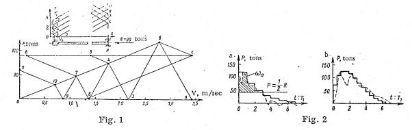
Fig. 1. Solution of the problem of impact driving of a pile by the method of characteristics.
