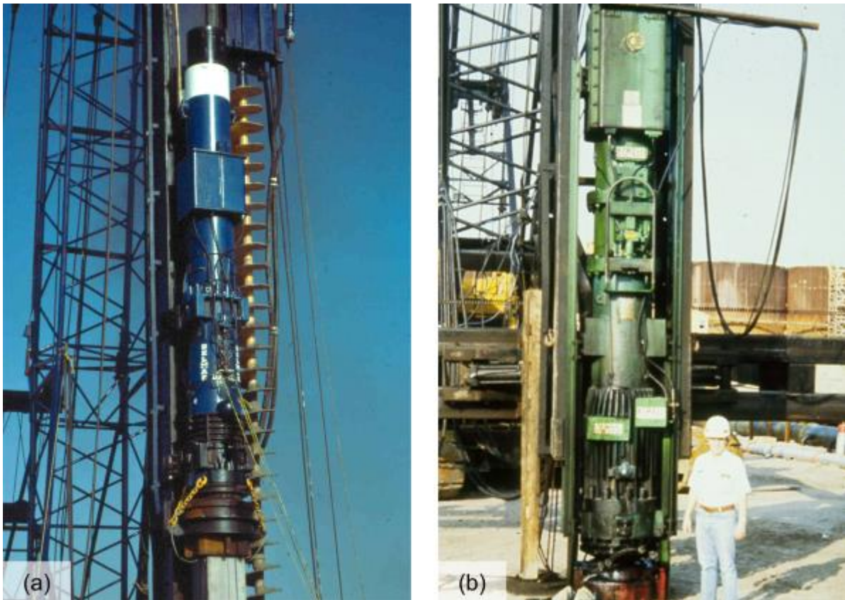
Figure 15-31 (a) Single acting diesel and, (b) double acting diesel hammers.
