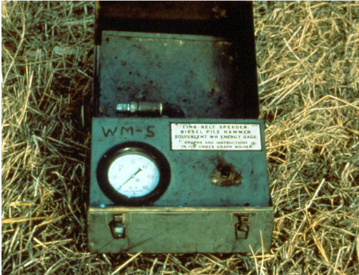
Figure 18-13 Typical external bounce chamber pressure gauge.
