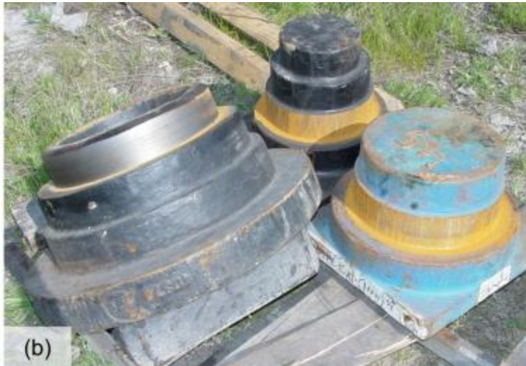
Figure 15-21 Inserts for (a) H-pile and (b) varying pipe pile diameter and wall thickness.
