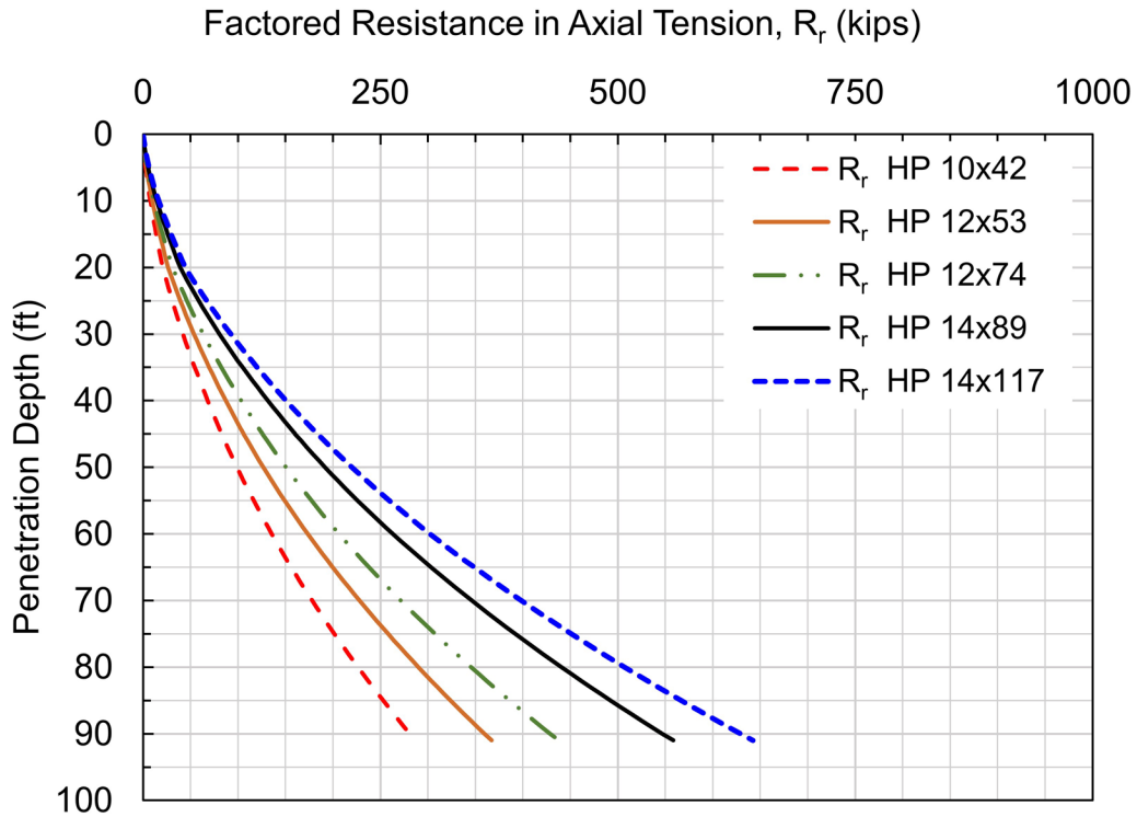
Figure D-17 Factored geotechnical resistance, R_r , in axial tension based on field determination by static load test, \phi_{dyn}=0.60 .
