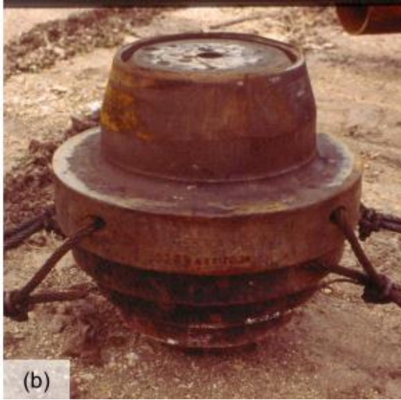
Figure 15-20 One piece helmets for (a) concrete pile and (b) pipe pile.
