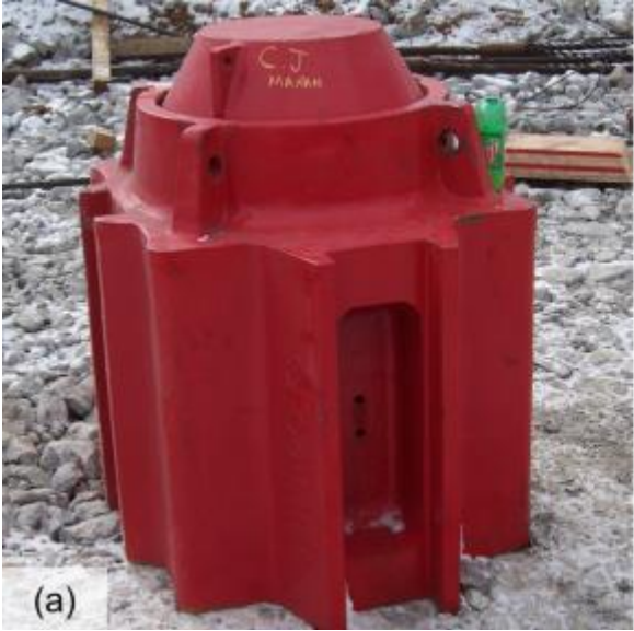
Figure 15-20 One piece helmets for (a) concrete pile and (b) pipe pile.
