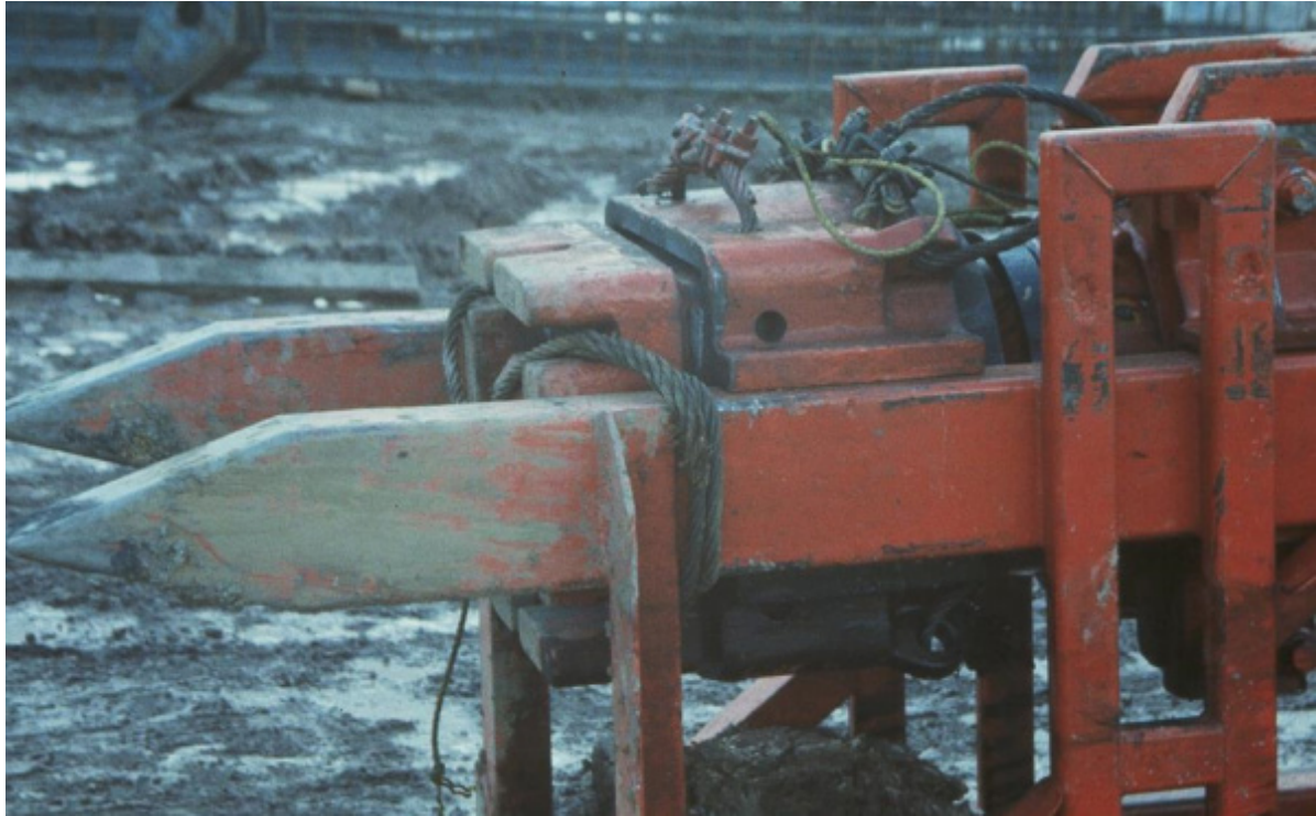
Figure 15-8 Stabbing guide at bottom of box leads.
