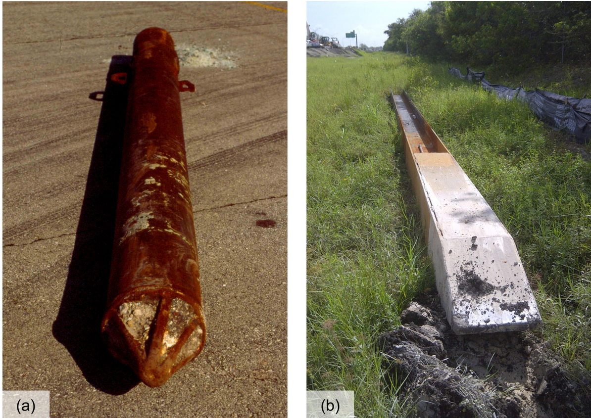
Figure 15-49 (a) Pipe pile and (b) H-pile spuds.
