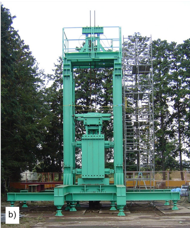
Figure 11-7 Drop weight rapid load test systems: (a) Fundex system (courtesy Foundation Constructors Inc.) and (b) Hybridynamic system.
