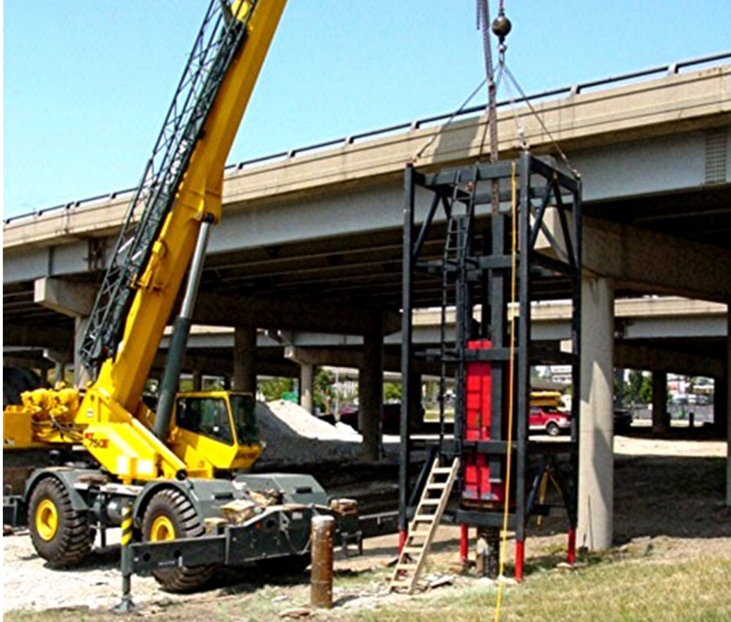
Figure 10-24 APPLE drop weight system.
