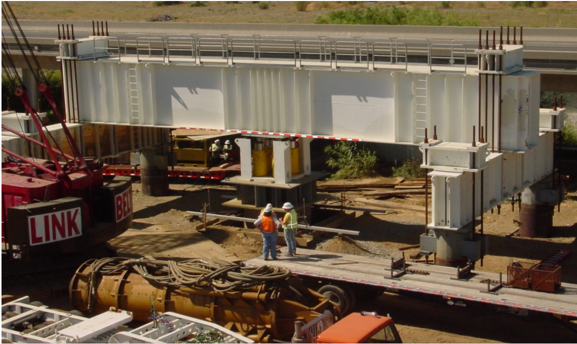
Figure 9-6 4000-Ton mobile load test frame (courtesy Caltrans).
