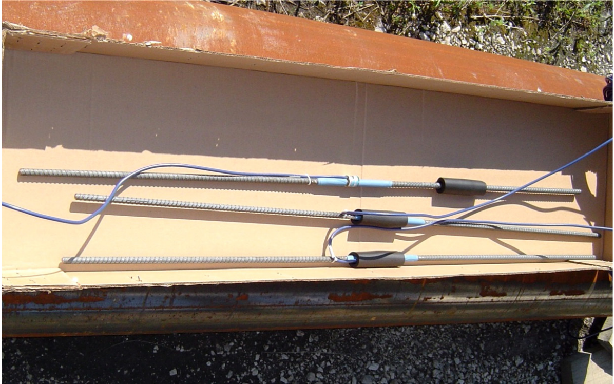
Figure 9-21 Vibrating wire strain gage sister bars for concrete embedment.
