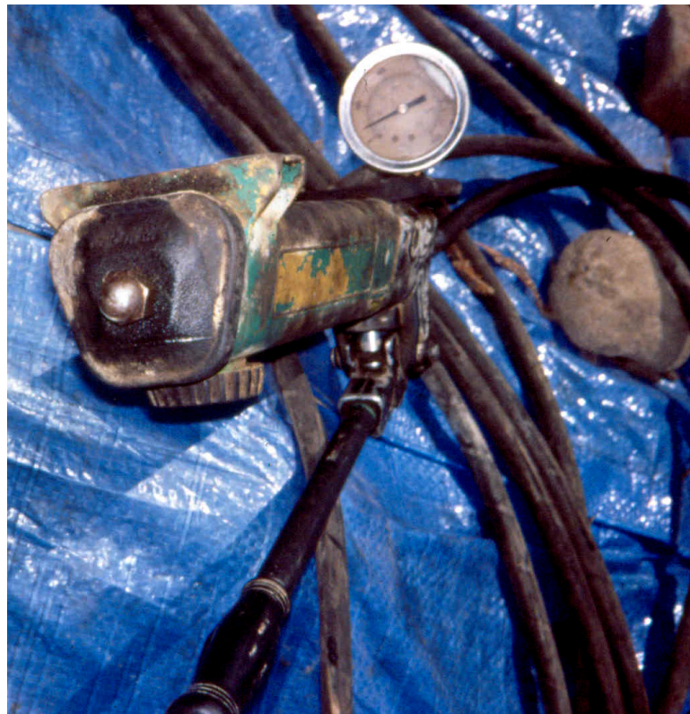
Figure 18-11 Hydraulic pump for fuel pump adjustments.
