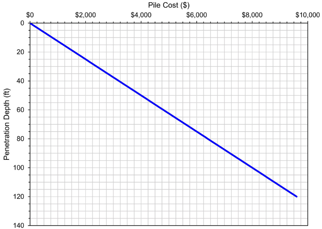
Figure 3-3 Pile cost versus pile penetration depth.
