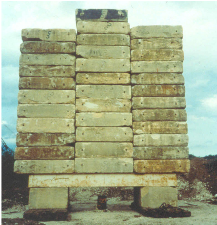
Figure 9-7 Static load test setup using weighted platform.
