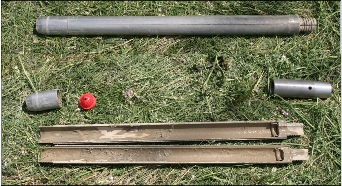
Figure 4-2 Standard split spoon sampler.
