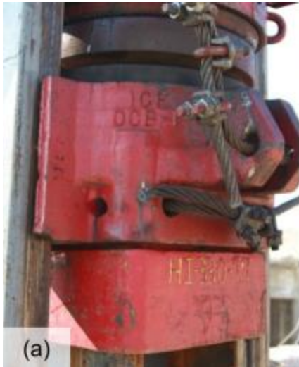
Figure 15-21 Inserts for (a) H-pile and (b) varying pipe pile diameter and wall thickness.
