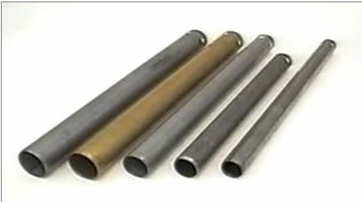
Figure 4-3 Shelby tubes (after Mayne et al. 2002).
