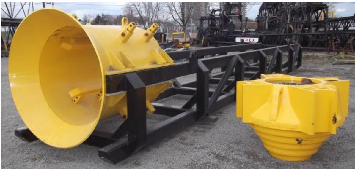
Figure 15-15 Offshore lead and pile guide (left) with pipe pile helmet (right) (courtesy Berminghammer).
