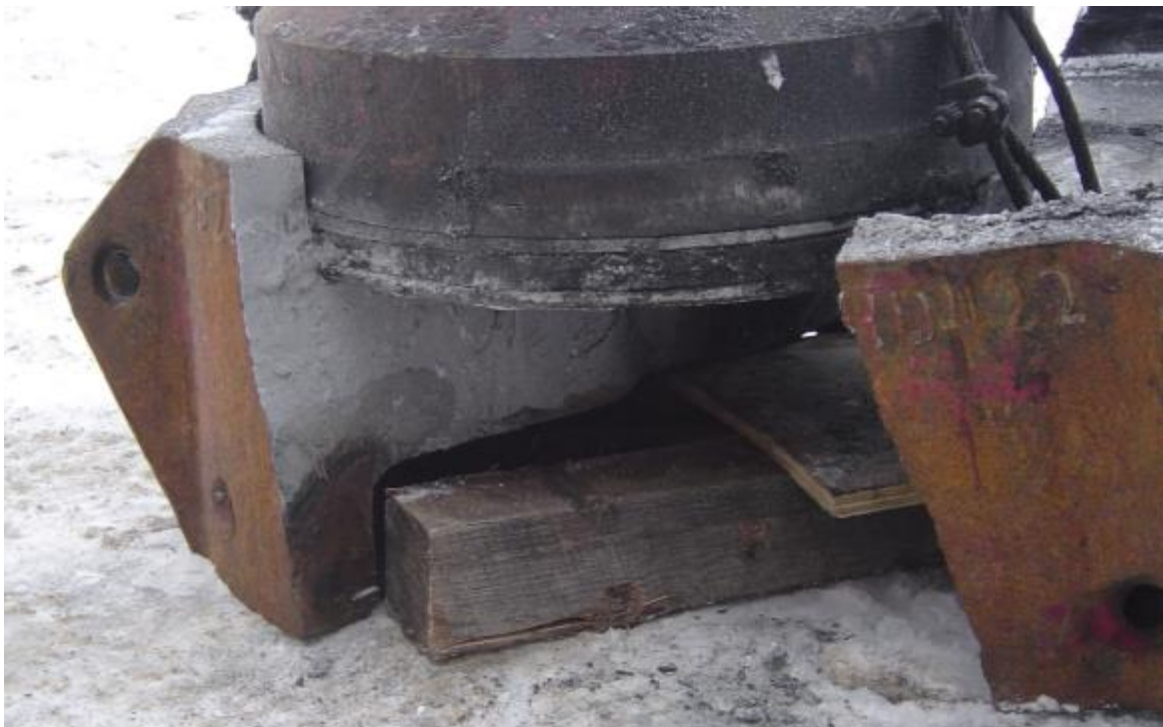
Figure 15-19 Cross section of cracked helmet with striker plate and aluminum and micarta hammer cushion (courtesy of WKG 2 ).
