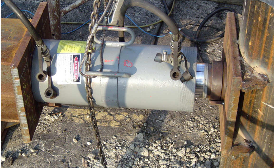
Figure 9-13 Jack for lateral load test (courtesy of WKG 2 ).
