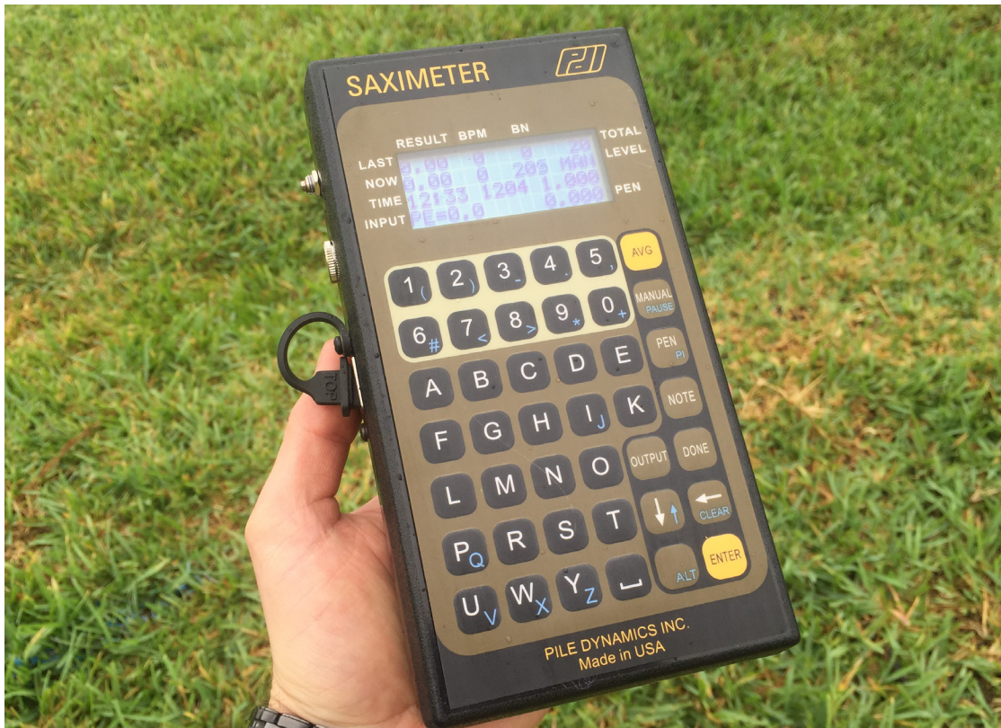
Figure 15-42 E-Saximeter wireless kinetic energy readout device.
