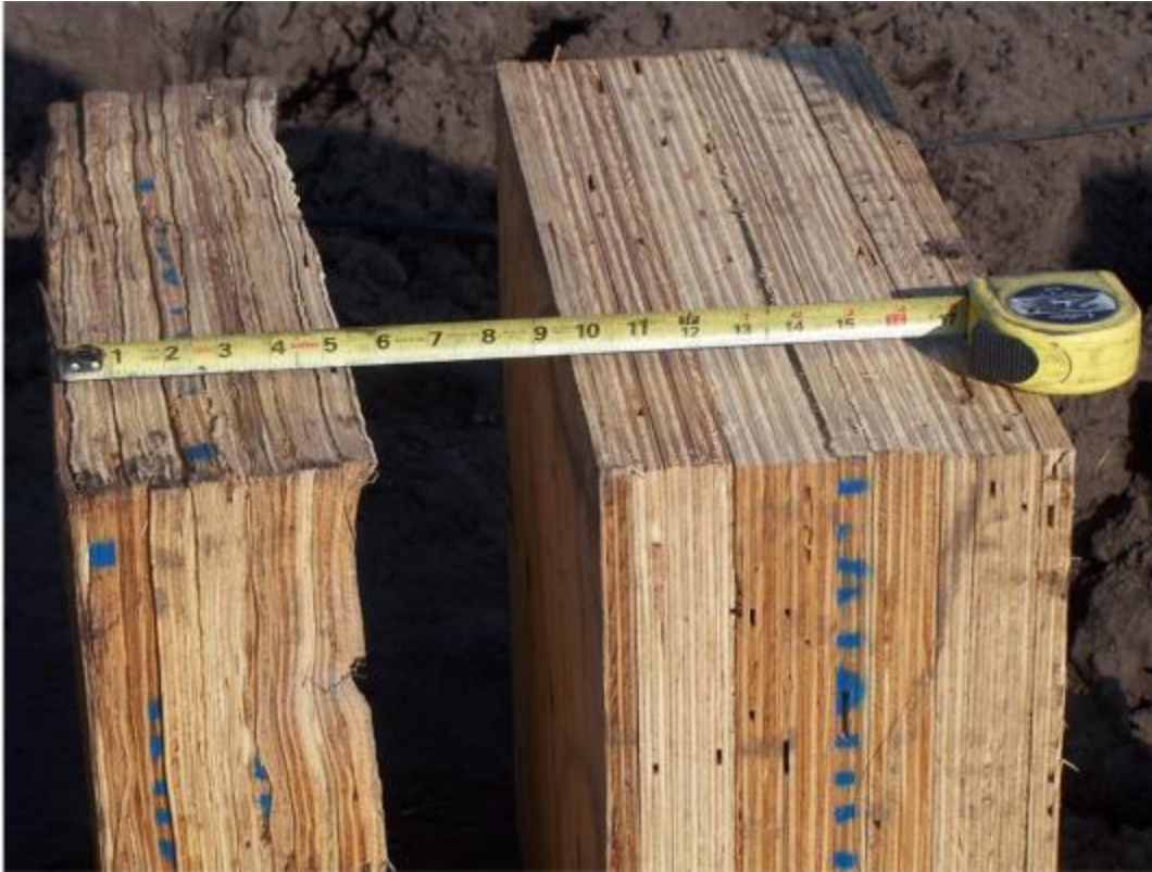
Figure 15-23 Plywood pile cushions: (left) used and (right) new.
