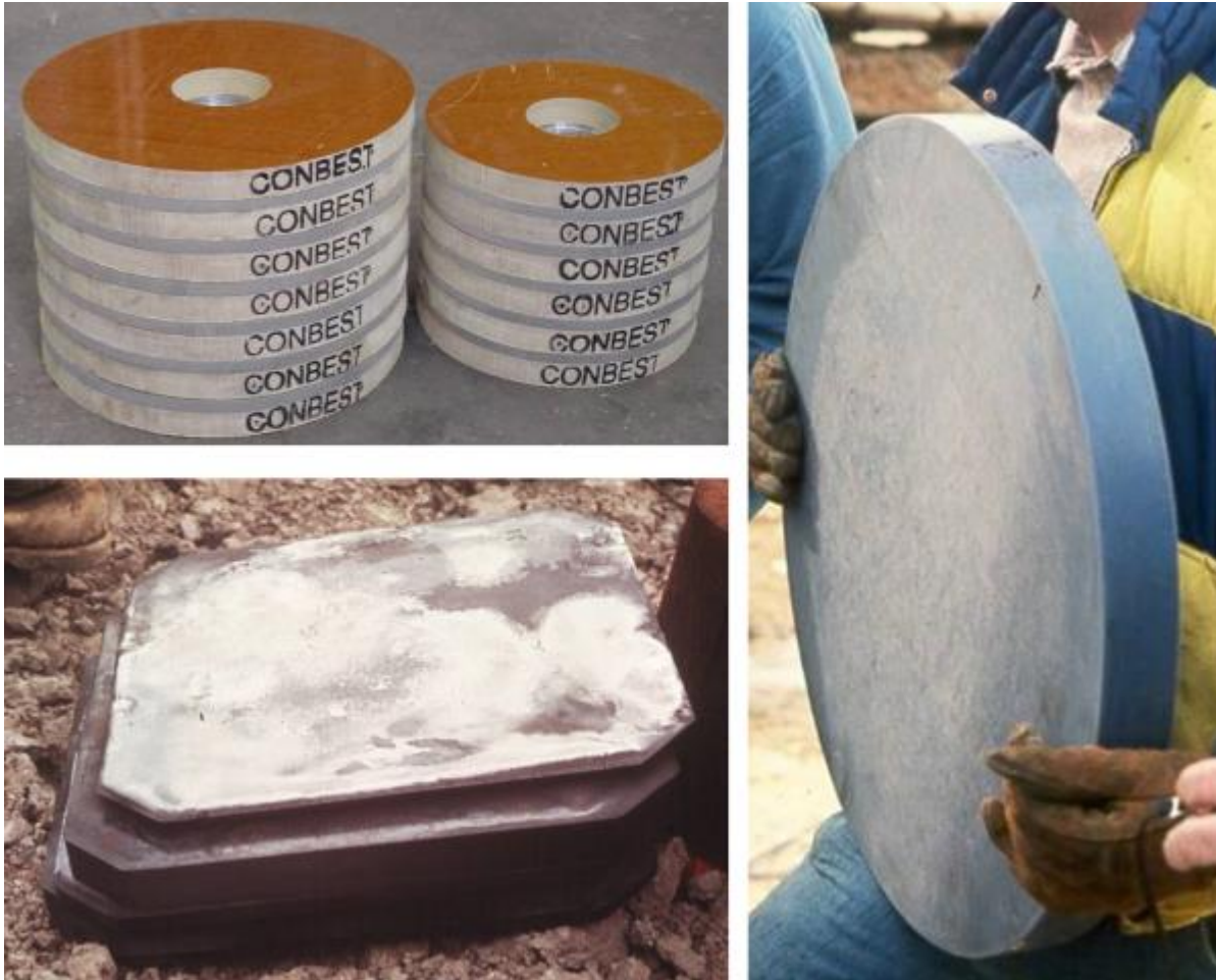
Figure 15-22 Typical hammer cushion materials.
