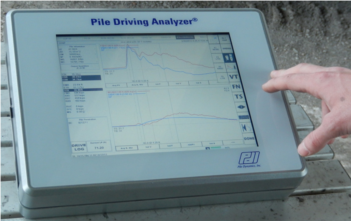
Figure 10-5 Pile Driving Analyzer processing unit (courtesy of Pile Dynamics, Inc.).
