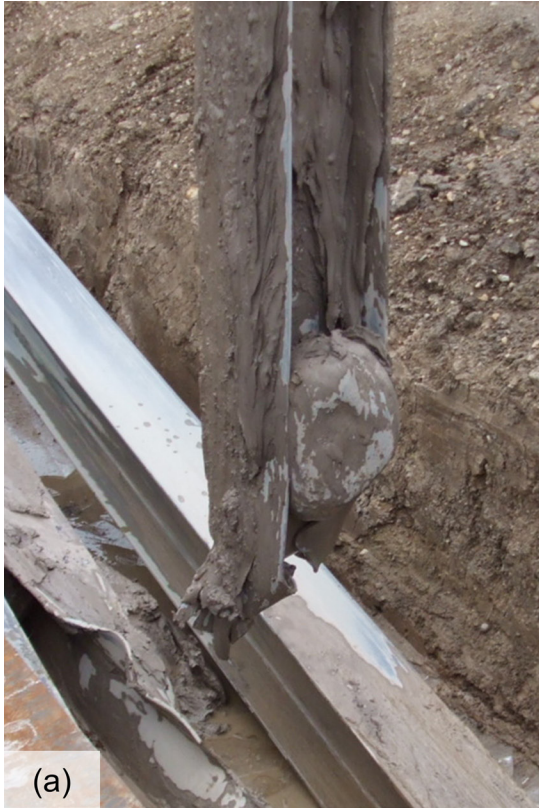
Figure 16-4 Damaged H-pile driven without pile toe protection (courtesy Wisconsin DOT).
