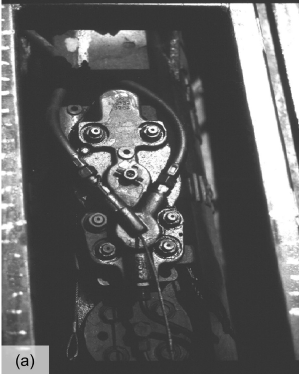
Figure 18-10 Fuel Pumps: (a) fixed four step pump and (b) variable fuel pump.
