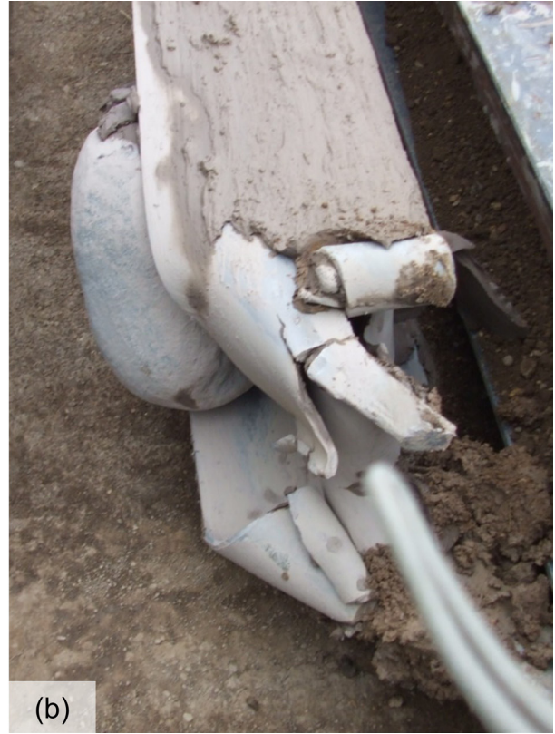
Figure 16-4 Damaged H-pile driven without pile toe protection (courtesy Wisconsin DOT).
