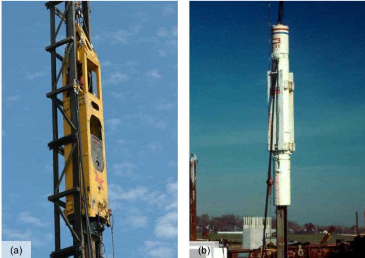
Figure 15-34 (a) Single acting hydraulic, and (b) double acting hydraulic hammers.
