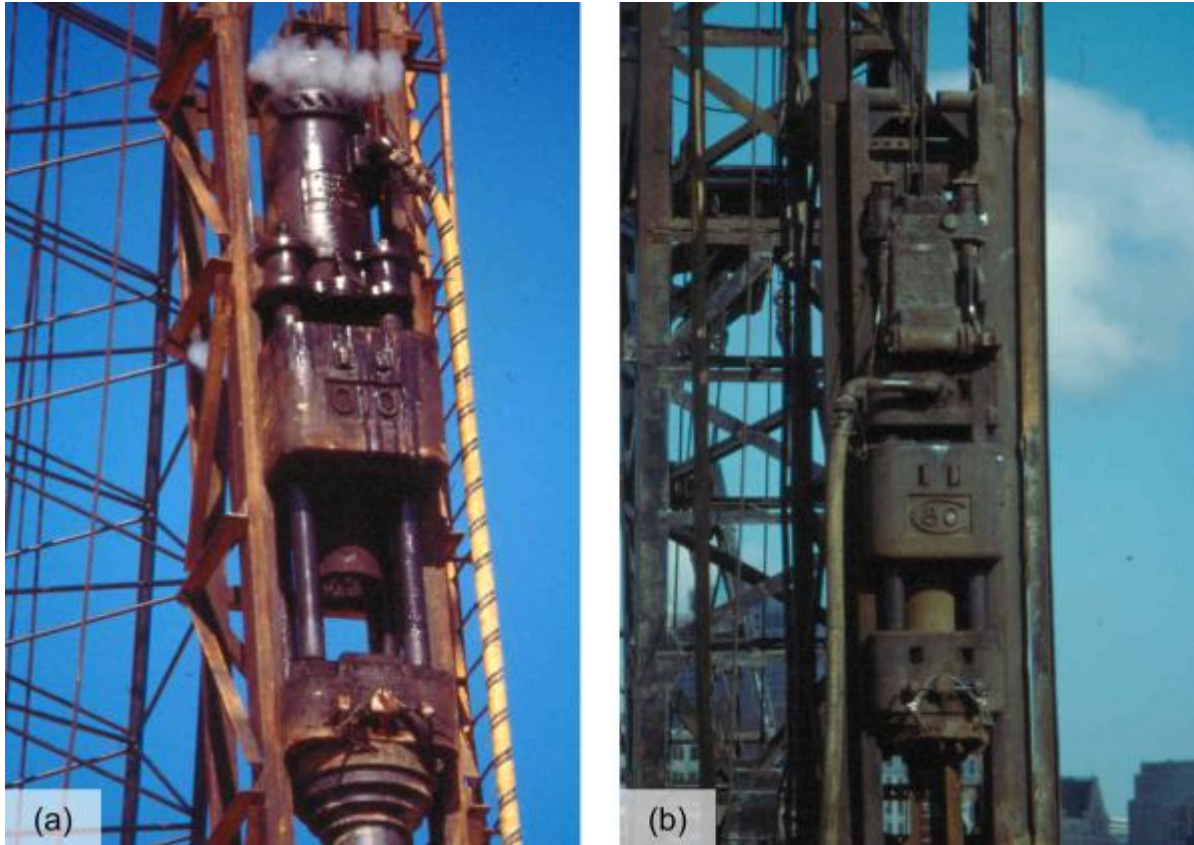
Figure 15-27 (a) Single acting air, and (b) differential acting air hammers.
