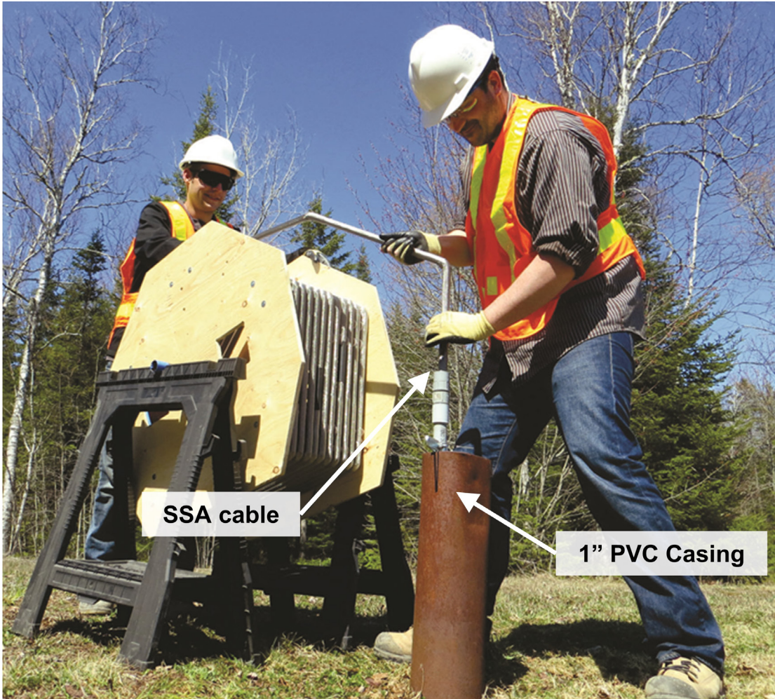
Figure 9-16 Typical Shape Accel Array (SSA) (courtesy of Measurand).
