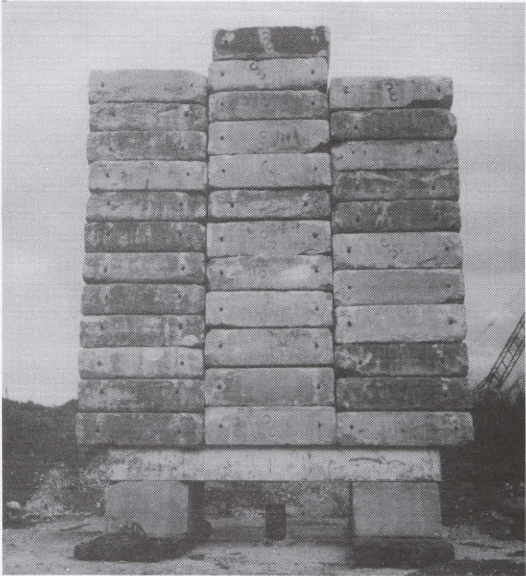
Figure 19.4 Typical Compression Load Test Arrangement using a Weighted Platform
