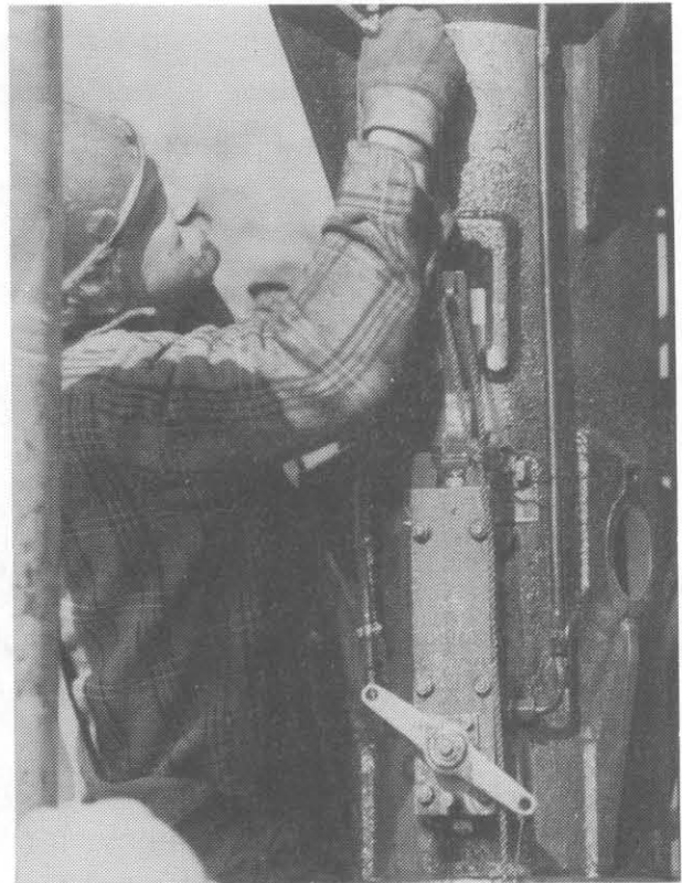
Figure 24.9 Variable Fuel Pump on FEC Hammer
