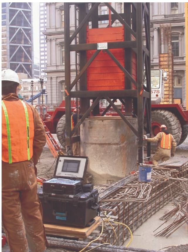
Figure 3. Dynamic load test of a drilled shaft using a 356 kN drop weight.
