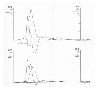
Figure 5. PDA's result for pile number p182
