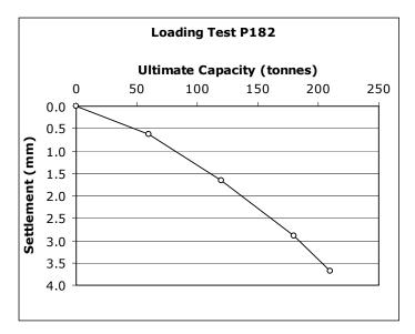
Figure 4. Result of static loading test
