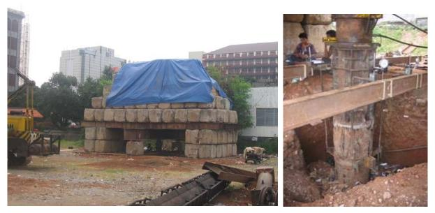
Figure 3. Loading test on progress (left) Cracks on pile during loading test (right)
