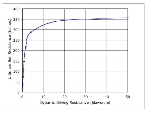
Figure 6. Bearing capacity graph for pile number P182
