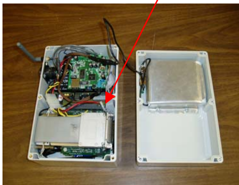
a) Remote Data Acquisition Unit
