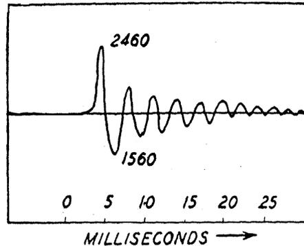
Figure 4 Recorded tension in the pile midpoint (in psi, after Glanville et. al. (1938))
