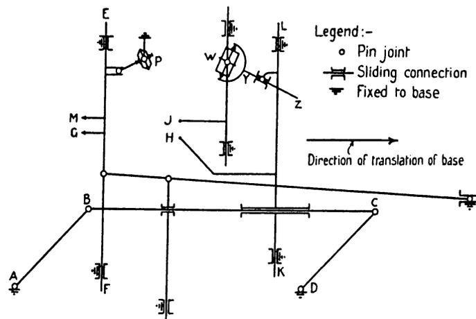
Figure 2 Graphical Machine for Wave Equation Solution (after Isaacs (1931))
