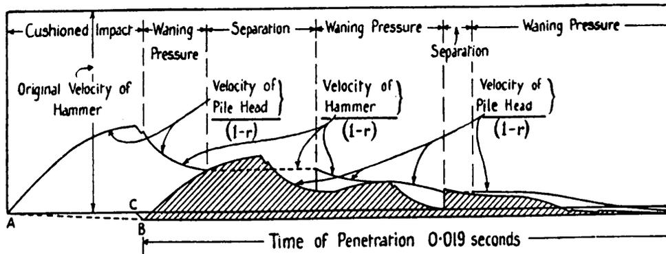
Figure 1 Graphical Solution of the Wave Equation (after Isaacs (1931))
