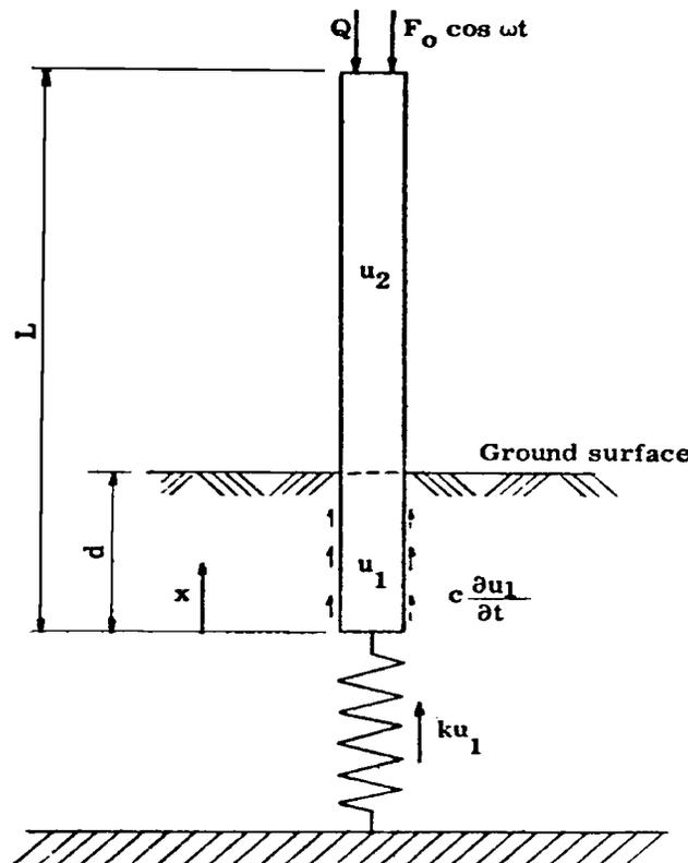
Figure 5 Diagram of Pile Model (after Hejazi (1963))
